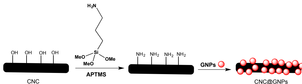
Figure 6-3: Schematic illustration of synthetic approach for making CNC@GNPs.
