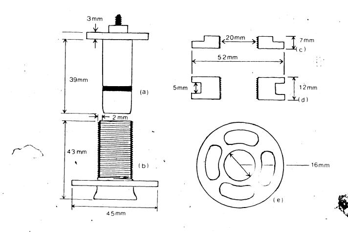
Figure App. -5.1 Nylon intestinal cannula and associated components:
