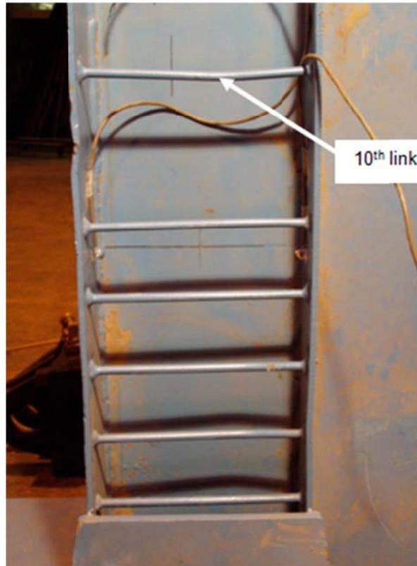
Figure 3-11: Link Initial Imperfections in South Column (East Side)
