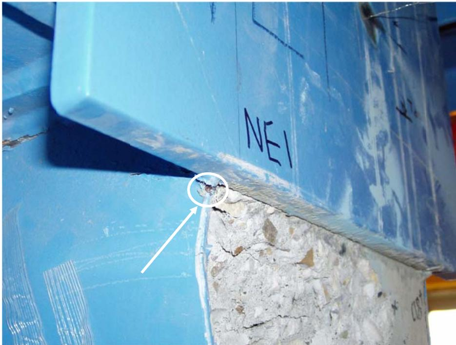
Figure 4-21: Flange Tear at Top of Columns in Cycle 29
