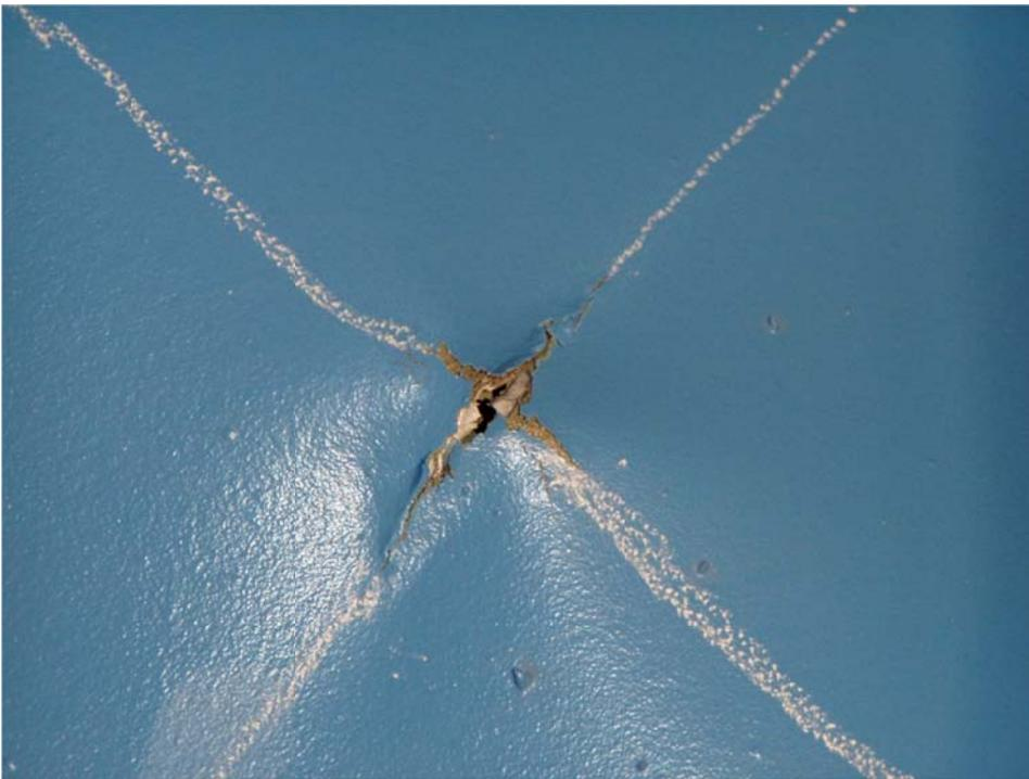
Figure 4-18: "S" Shaped Tear in Infill Panel in Cycle 25
