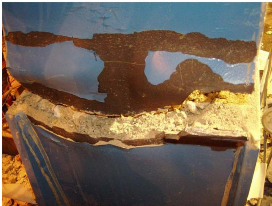
Figure 4-22: Flange Tear in Columns in Cycle 30
