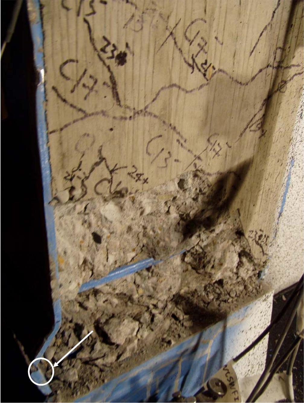
Figure 4-16: Tear at Crest of Buckled North Flange in North Column in Cycle 26
