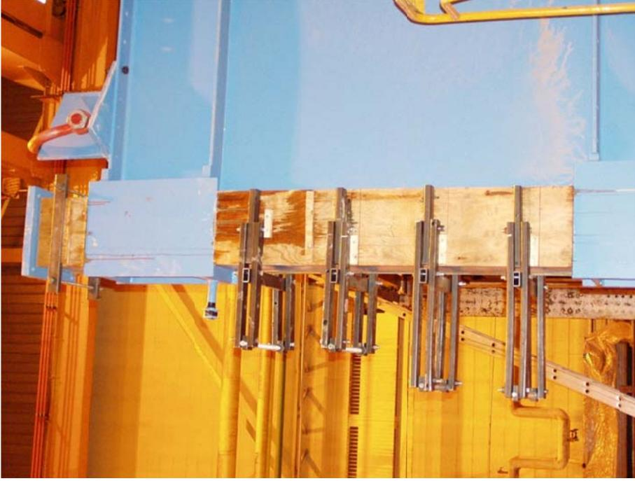
Figure 3-6: Concrete Casting and Formwork Arrangement
