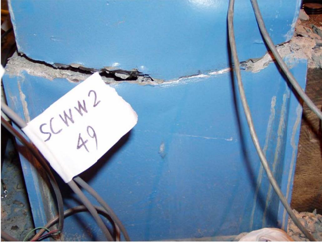
Figure 4-15: Opening in South Flange of South Column in Cycle 25
