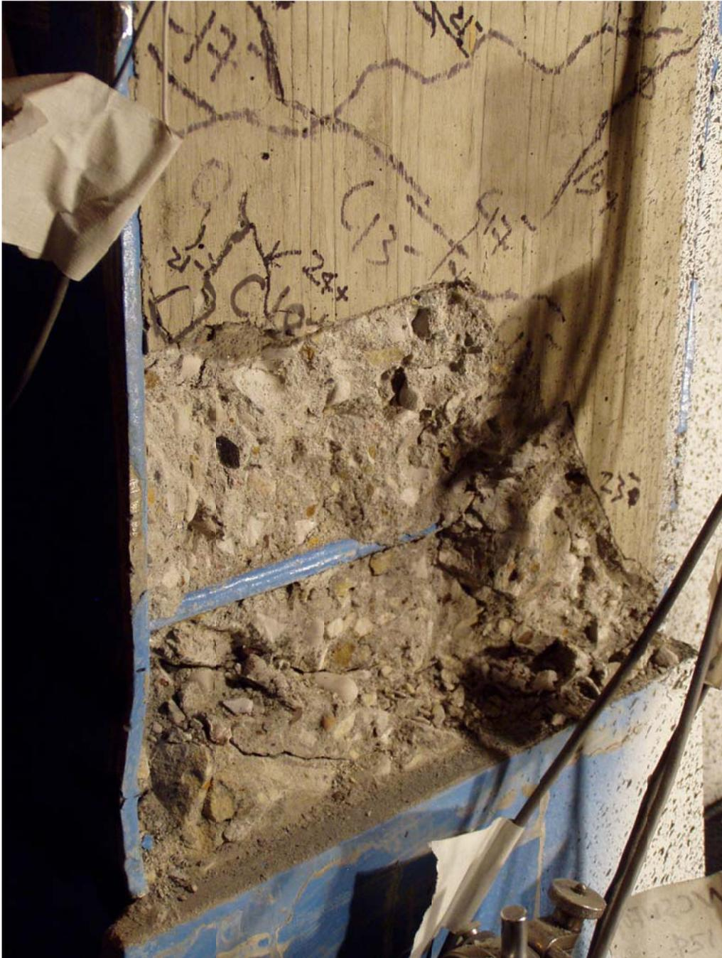
Figure 4-14: Link Exposed in West Side of North Column in Cycle 24
