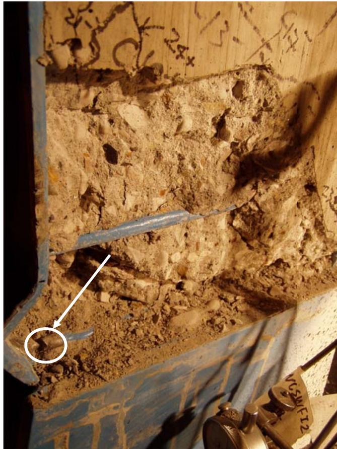
Figure 4-17: Link Torn from Column Flanges in Cycle 26
