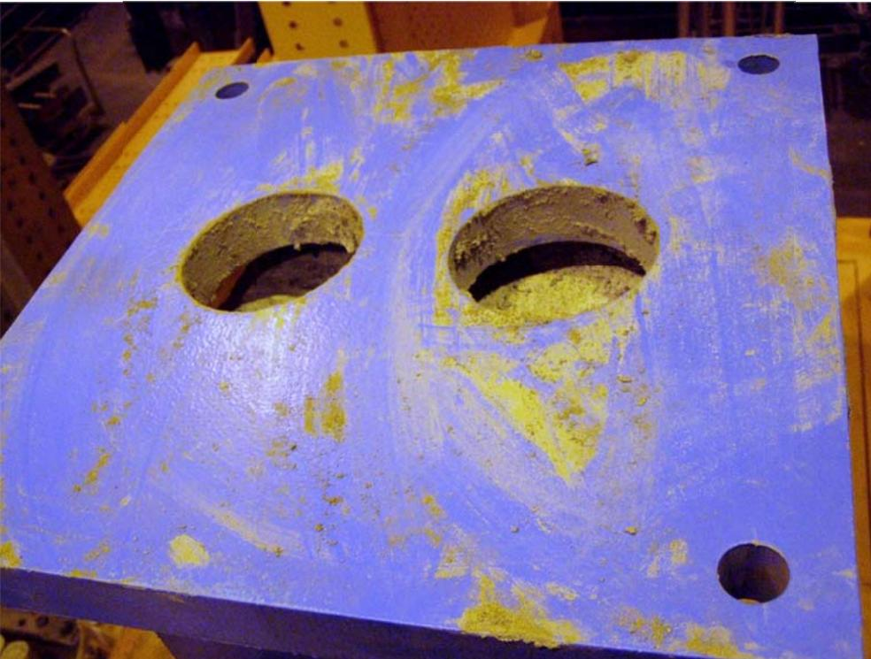
Figure 3-7: Gap Left at Top of Columns for Grouting
