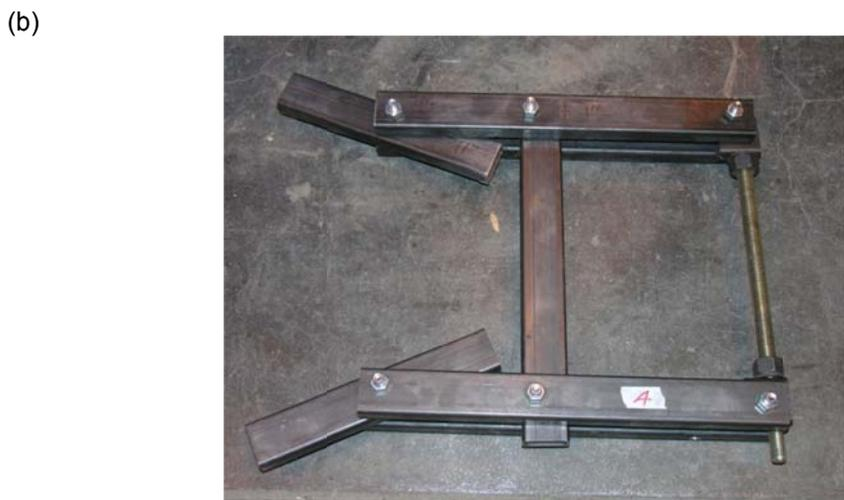
Figure 3-8: Formwork Clamp
