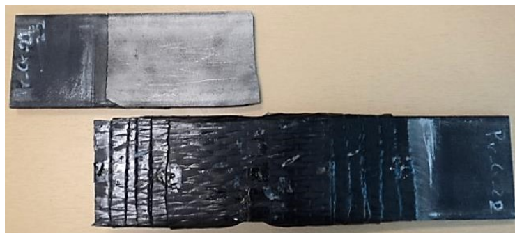
Figure 5.115 Delaminated CFRP surface and the failed specimen 9-SKWRP-Sk300-B
