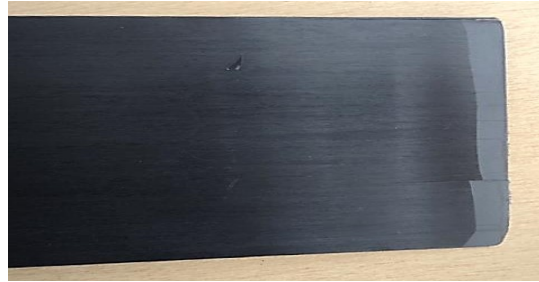
Figure 5.8 Tapered end of Sika Carbodur formed by grinding
