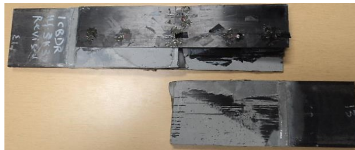
Figure 5.35 Delaminated CFRP surface and the failed specimen 1-CBDR-Half-Th-Sk-30
