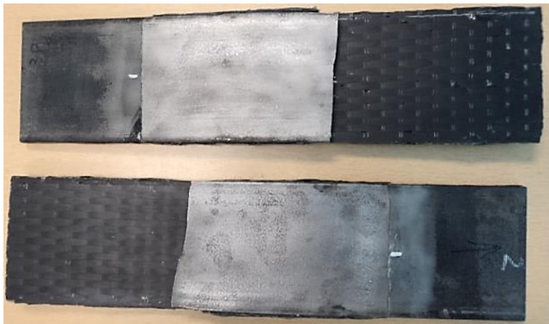
Figure 5.84 Delaminated CFRP surface and the failed specimen 6-SKWRP-Sk-300-B
