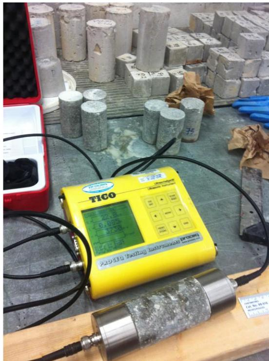
**Figure 3-5 Test setup for UPV**
