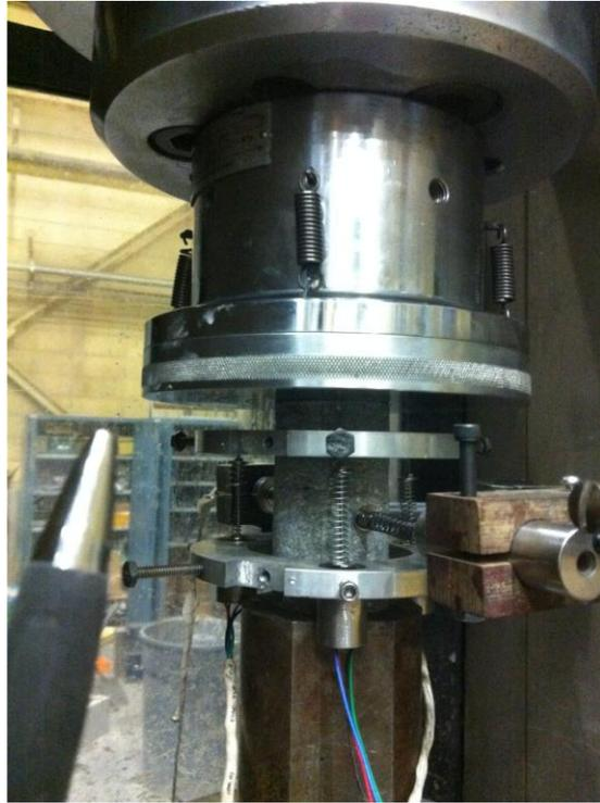
**Figure 3-4 Test setup for modulus of elasticity**
