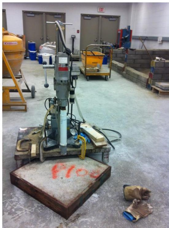
**Figure 3-3 Coring machine for the sample drilling**
