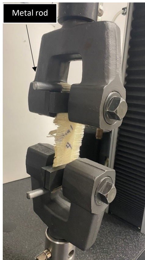
Figure 27. Tensile strength test for Fabric U, using a long specimen length wrapped around and a metal rod outside the upper and lower clamps.
