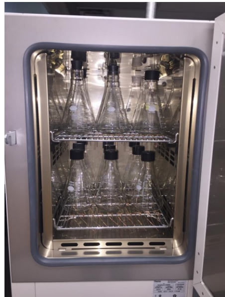
Figure 20. The positioning of flasks inside the oven.
