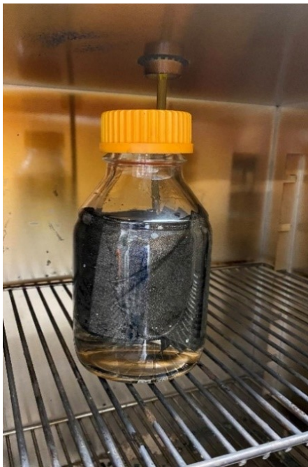
Figure 32. Reducing GO-coated specimens in L-AA.
