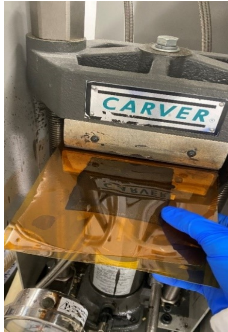
Figure 30. Drying of specimen using the heated press.
