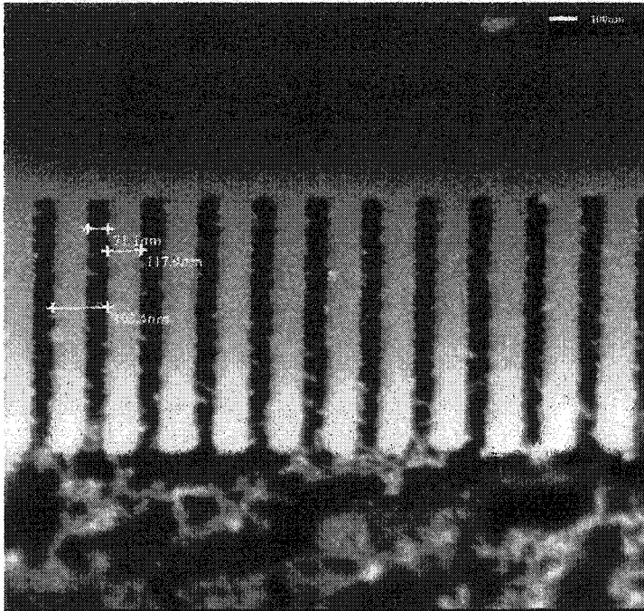
Figure 4.13: SEM picture showing a closer look at the grating fingers for grating pattern formed by a dose of 500 \mu\text{C}/\text{cm}^2
