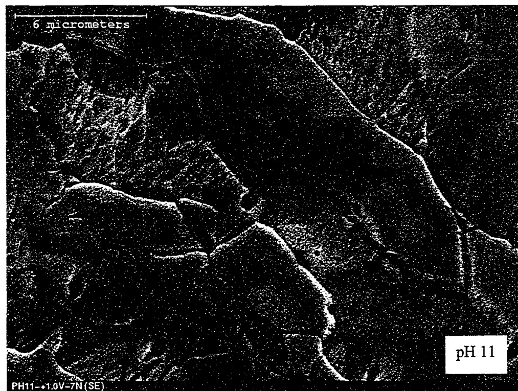
Figure 4-8. SEM micrographs of surfaces after corrosive polishing at different slurry pH under a potential of +1 V and a normal wearing load of 7 N.
