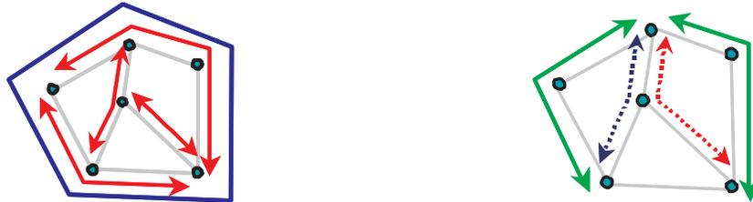
(i) FIPP protecting a set of span disjoint working routes      (ii) Non-disjoint paths sharing the same FIPP
