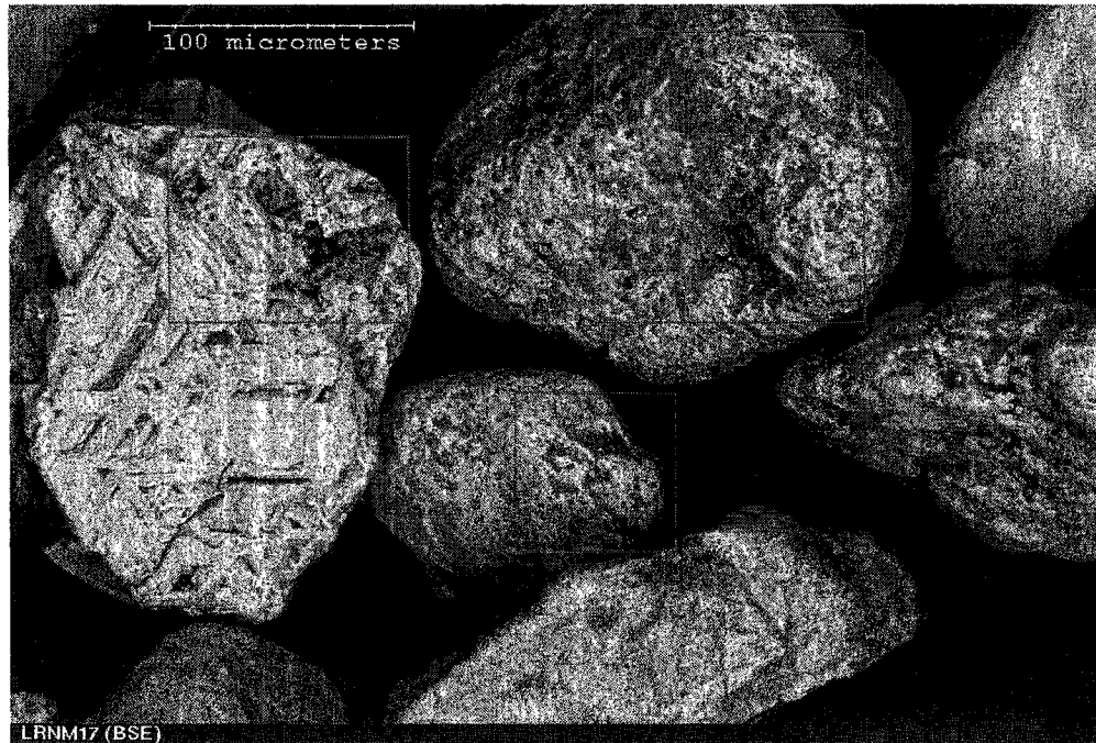
Figure 31 A typical SEM image of the rutile concentrate. The marked areas show embedded darker grains, which are siliceous minerals. The smooth crystal in the upper right corner is pure rutile.
