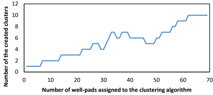
Fig. 5-16. Number of clusters during the clustering process. It shows how the clusters with a common well-pad merged.
