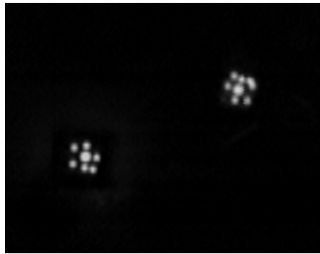
Figure 4.19: Raw vision data captured by Microsoft Surface when there are two tags on the tabletop
