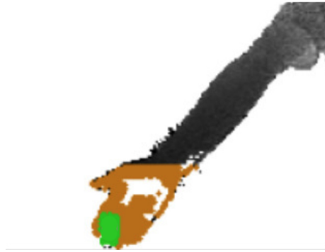
Figure 4.14: Hand detection when surface tabletop is turned on and the camera is mounted at the side of the surface, the white area is the data loss due to the interference.
