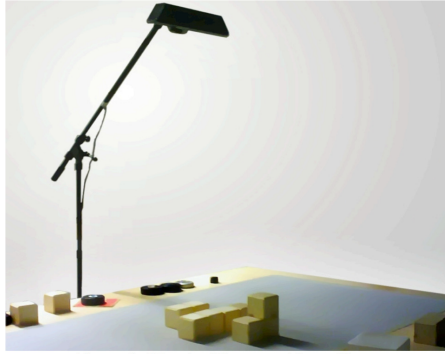
Figure 2.4: dSensingNI [45] setup with a tabletop and a depth-sensing camera, capable to track users fingers and multi-touch interaction
