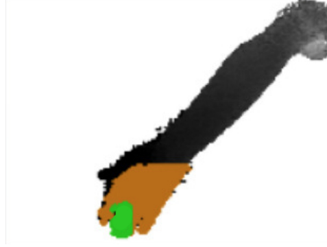
Figure 4.13: Hand detection when surface tabletop is turned off and the camera is mounted at the side of the surface
