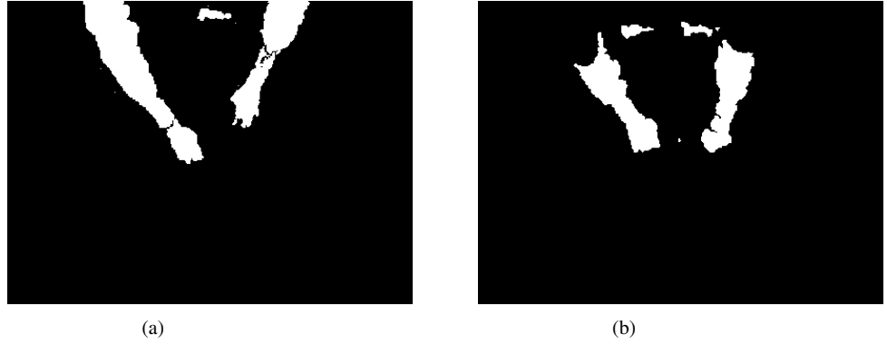
Figure 4.8: a) Depth map obtained from Kinect including the data of upper arms. b) Depth map obtained from Kinect losing the data of upper arms
