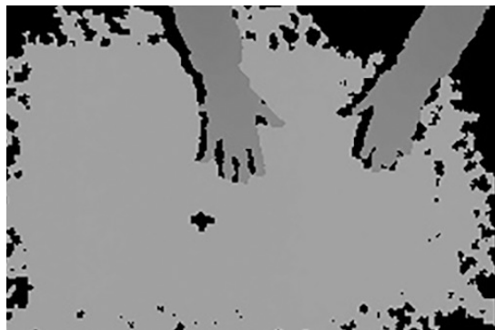
Figure 4.2: Depth images obtained from Kinect when the tabletop is turned off
