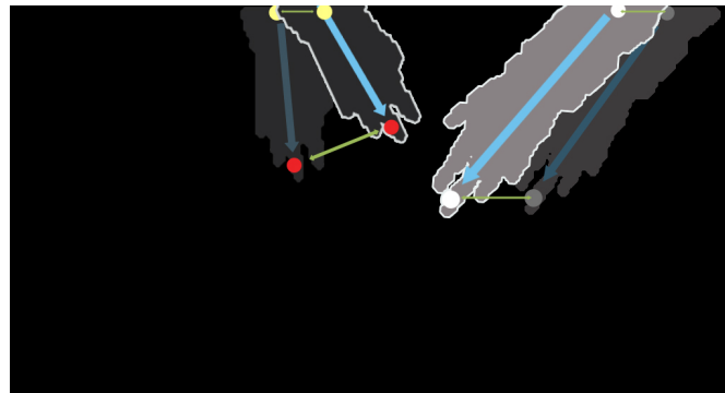
Figure 4.7: The comparison of distance between elbows and fingers when hands are moving, we can see that the moving distance of fingers are much longer than that of elbows.
