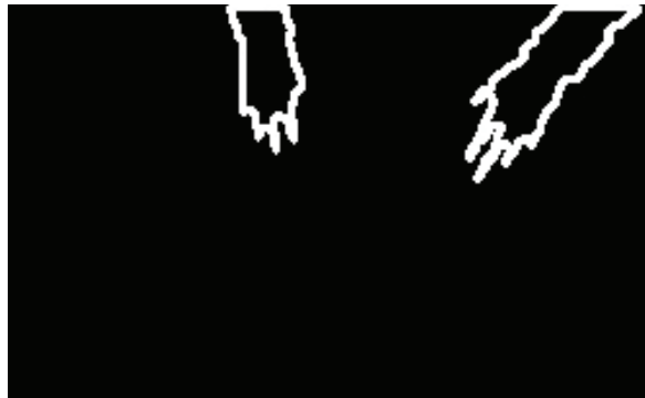
Figure 4.5: Contours found in depth image after noise elimination
