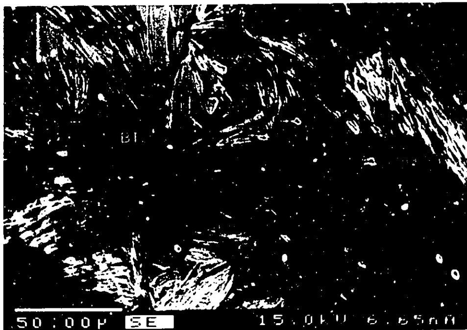
Plate 10. Secondary electron image of hematite in a quartz-biotite matrix. Note at the centre of the photo the platelet-like nature of the hematite. Scale bar represents 50 \mu m.
