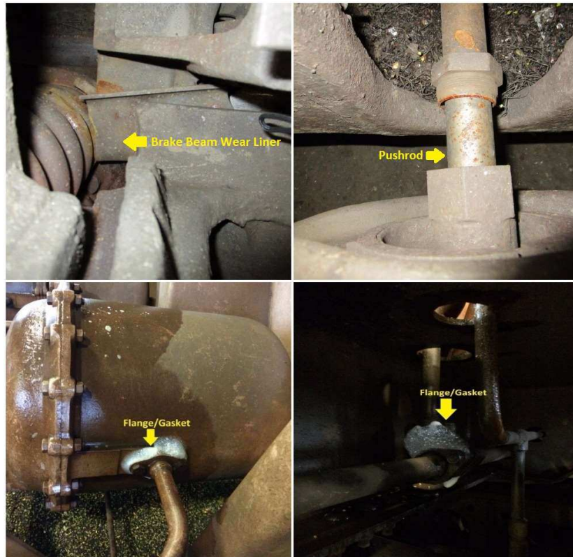
Figure 26. Grain Hopper Railcar Defects (multiple railcars) (Canadian Pacific, 2017) & (Photos by author)
