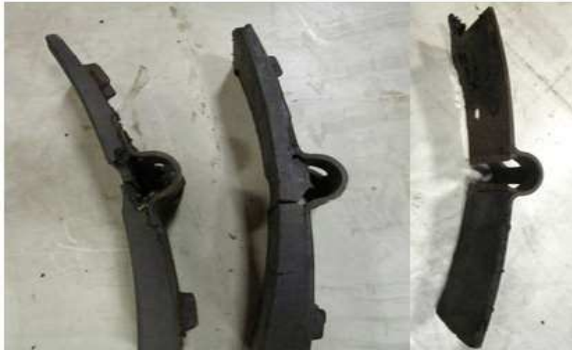
Figure 25. Worn out brake shoes (Canadian Pacific, 2017)
