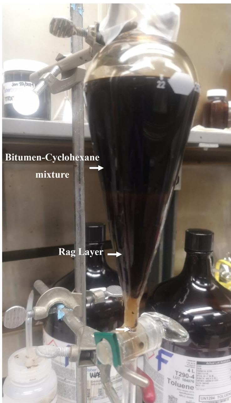
**Figure 4-2.** Set up of liquid-liquid extraction process using cyclohexane.
