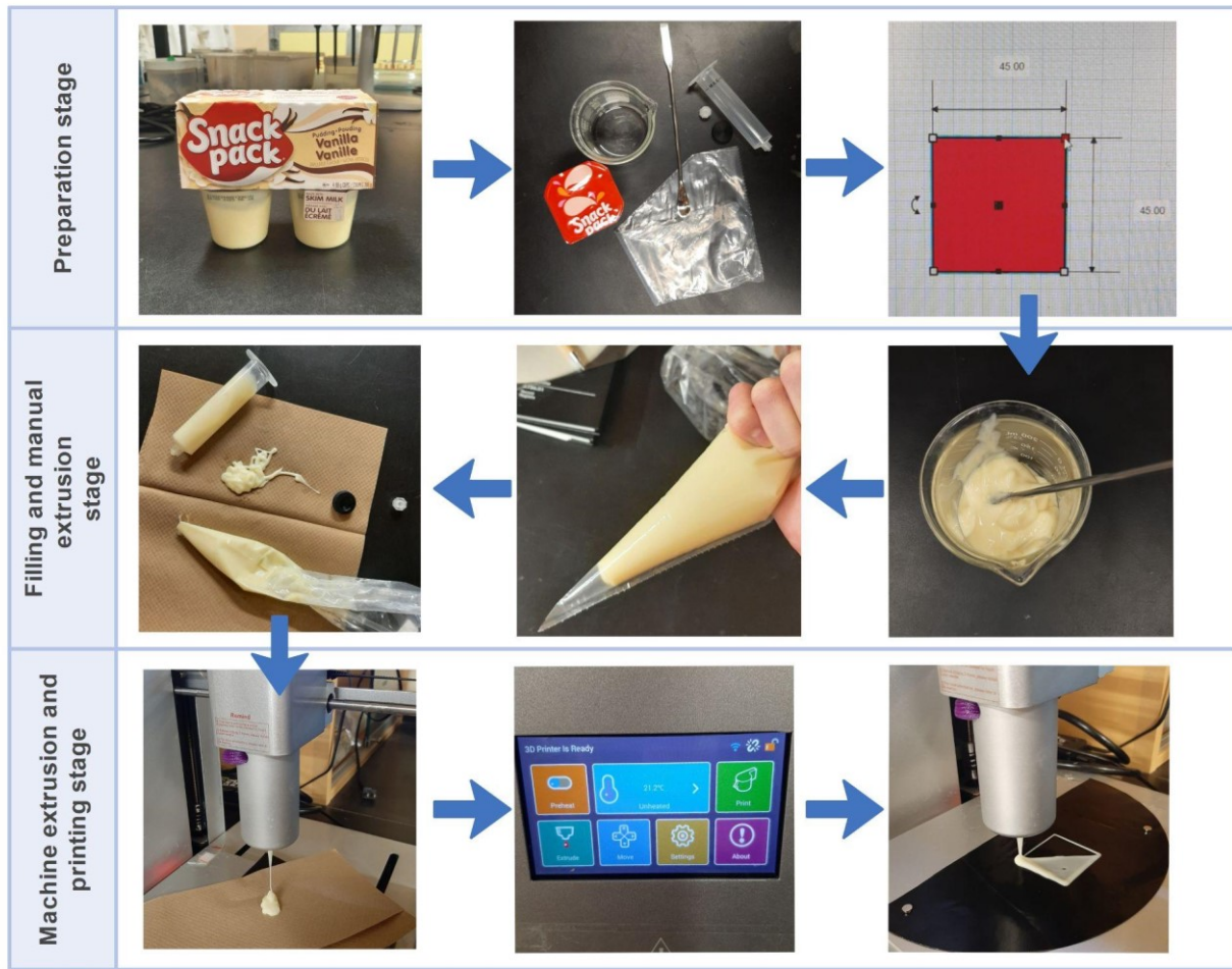
Figure 4. Diagram of a 3D food printing process from product selection to printing used in this study.
