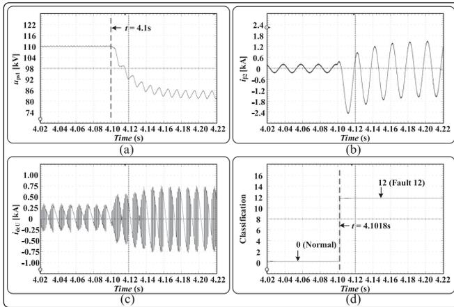
Fig. 11. Oscilloscope transient waveforms in scenario of *Fault 5* for: (a) AC TSS input three-phase RMS voltage, (b) ATR1 output current, (c) output current of rectifier of up vehicle, (d) output classification of the monitoring system.
