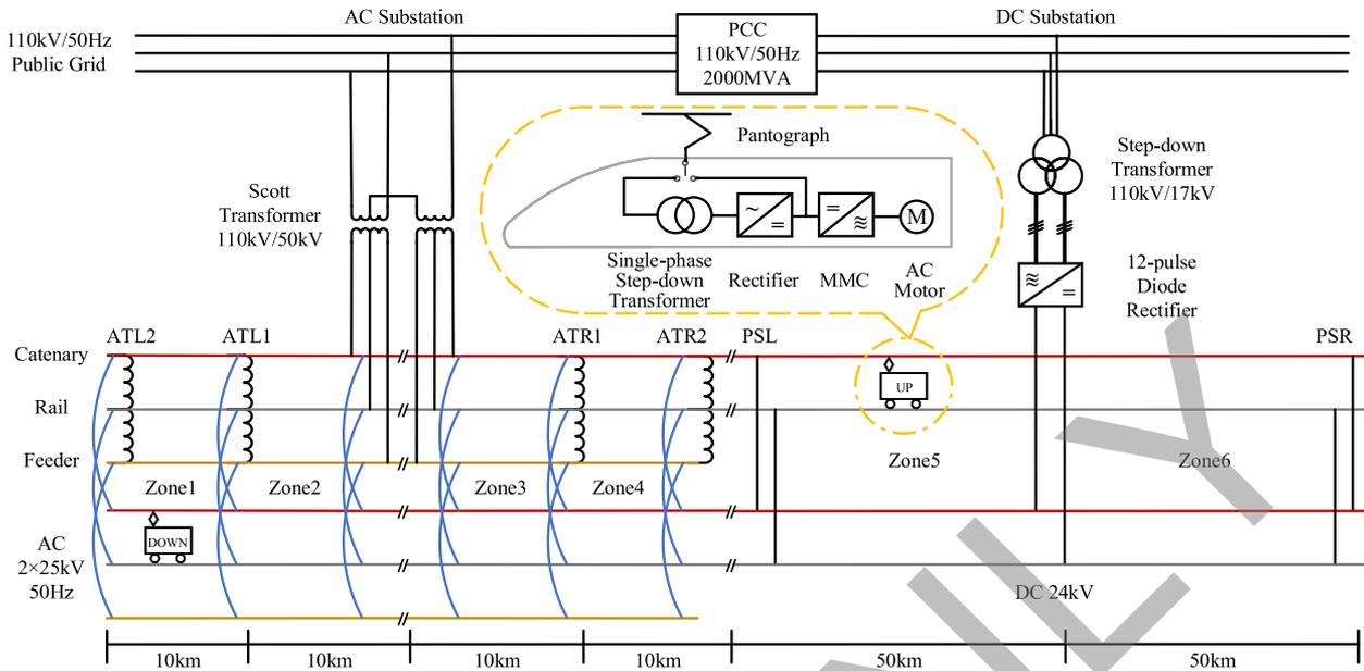
Fig. 1. Schematic of high-speed railway system under hybrid AC/DC grid.
