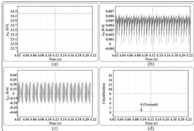
Fig. 15. Oscilloscope transient waveforms in scenario of *Normal Condition* for: (a) DC TSS output voltage, (b) PSR input current, (c) output current of rectifier of up vehicle, (d) output classification of the monitoring system.
