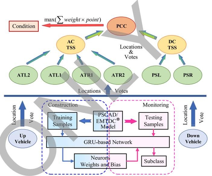
Fig. 4. Hierarchical structure of the monitoring system for FDI in HSR used in the off-line experiment.
