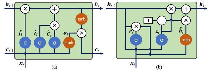
Fig. 3. Cell structures of standard LSTM and GRU. (a) LSTM. (b) GRU.
