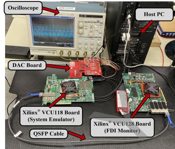
Fig. 9. Hardware emulation platform for real-time FDI experiment.
