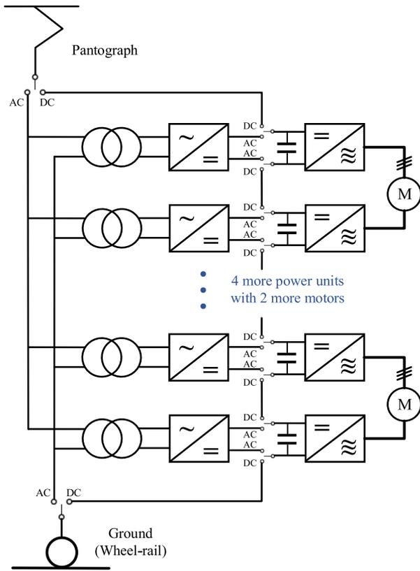
Fig. 2. Switch scheme for the vehicle operating under hybrid AC/DC grid.
