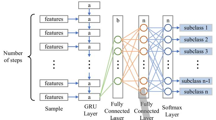
Fig. 5. Architecture of GRU-based network in sub-monitors for FDI in HSR.
