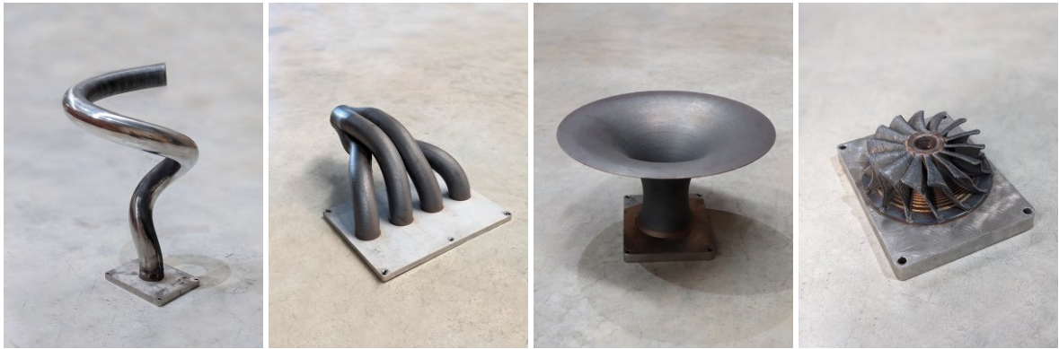
Fig. 1.2: Additively manufactured components using an LMD robot-based system [13].
