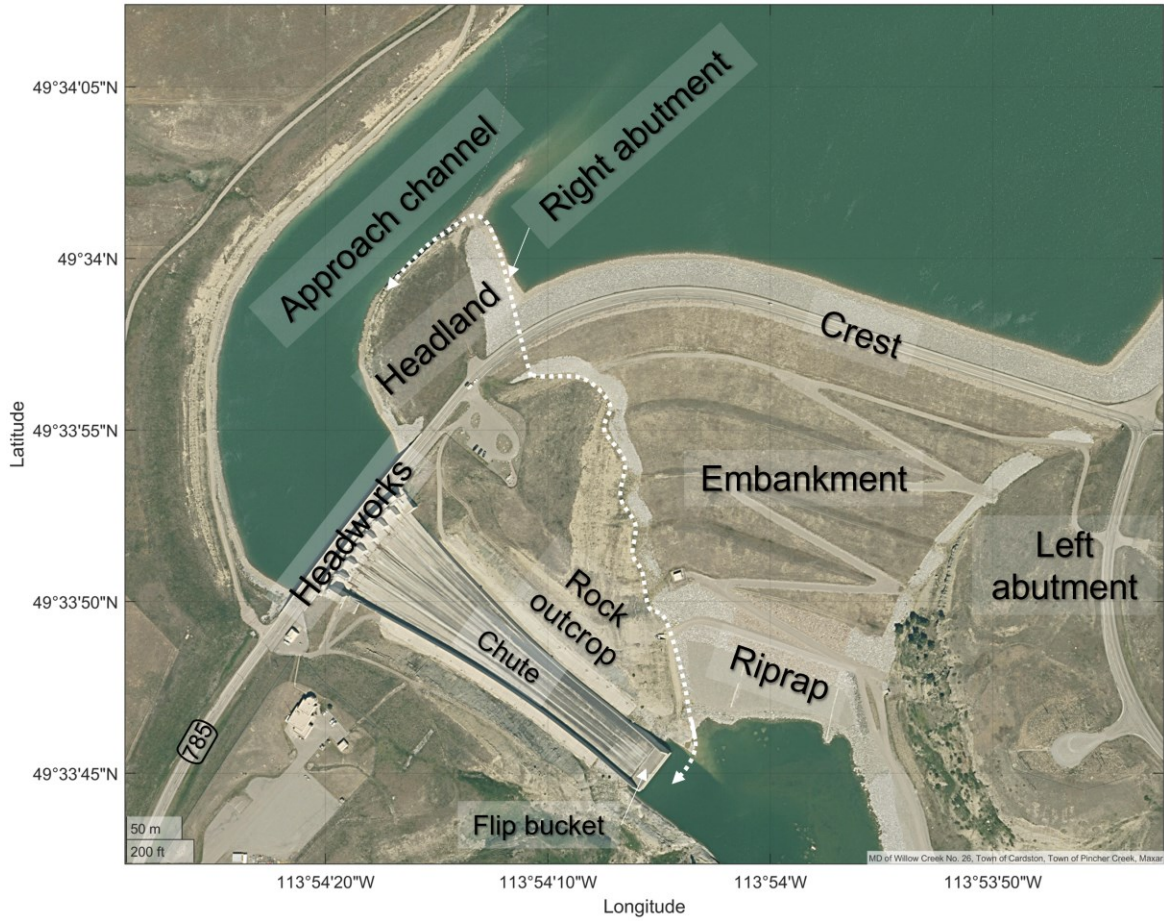
Figure 5- 1. Layout of different areas and elements of the ORD
