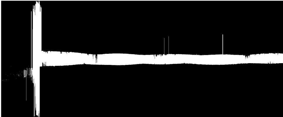
Figure 2.9: Resulting image when pixels between the edges along the height were marked white.
