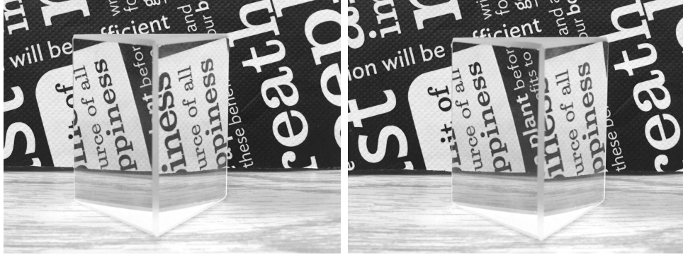
Figure 1.1: A transparent prism observed at two different viewpoints. Notice that the same surface point of the prism has different colors at the two viewpoints, making the color appearance being an unreliable cue for correspondence-based 3D reconstruction of transparent objects.
