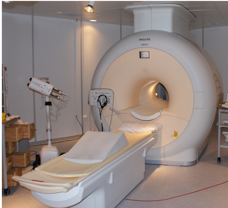
Figure 1.6: MRI Machine. Image of a Philips MRI machine. Visible in the image are the table which the patient lies on, the bore through which the table moves for imaging, and the casing containing the magnets. Image taken from [34].
