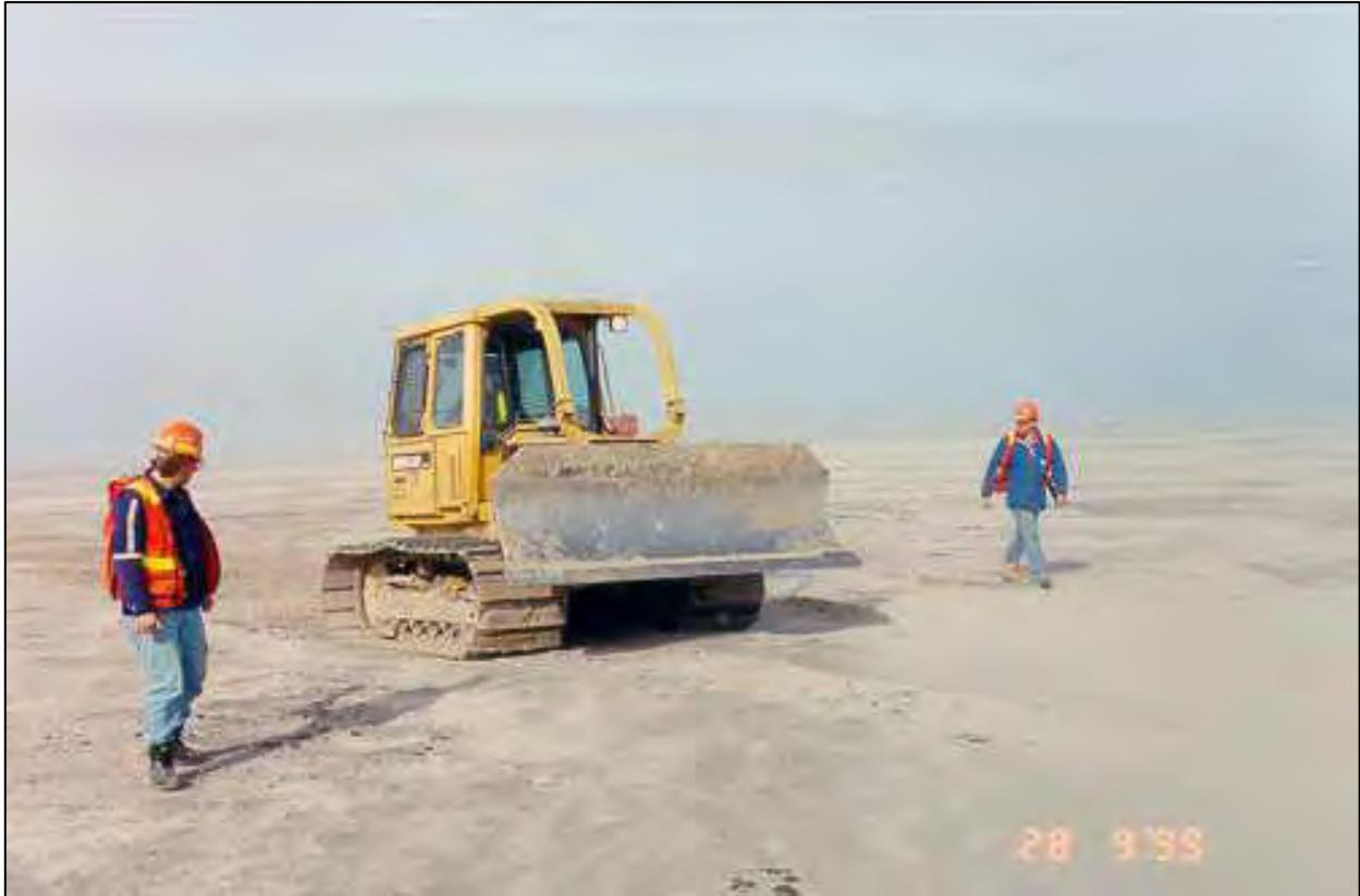
**Figure 3-10.** Trafficability testing with a Cat D3 dozer on the sand-capped CT Prototype in 1999.
