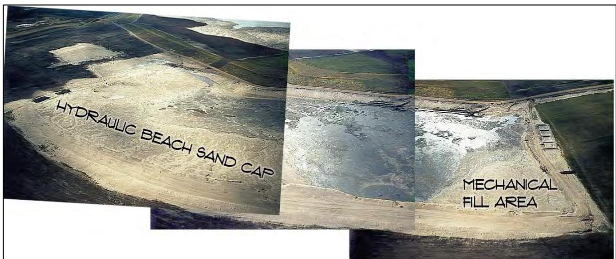
Figure 1-3. Syncrude CT Prototype shortly after sand-capping.
