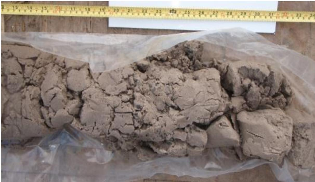
**Figure 3-1. Sonic drilling core of tailings sand from the foundation zone underlying Sandhill Fen (Fall 2008)**
