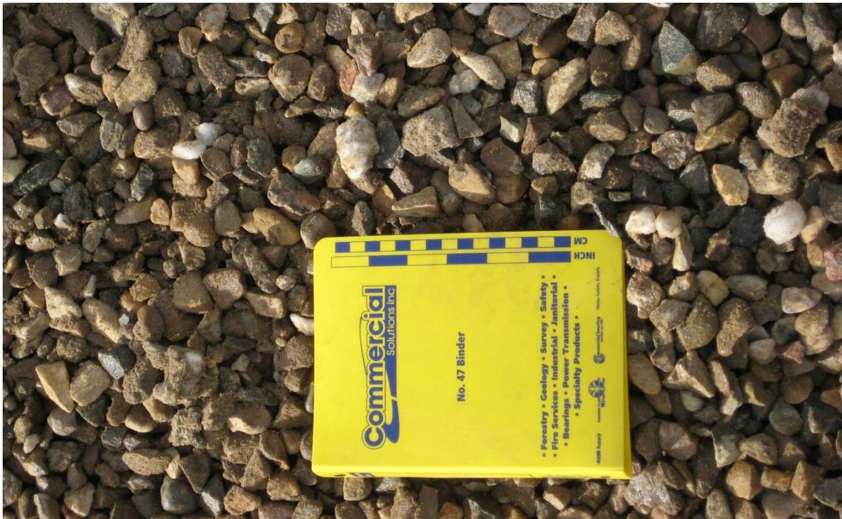
Figure 3-7. Crushed Gravel used as Sump Vault base (April 2009)
