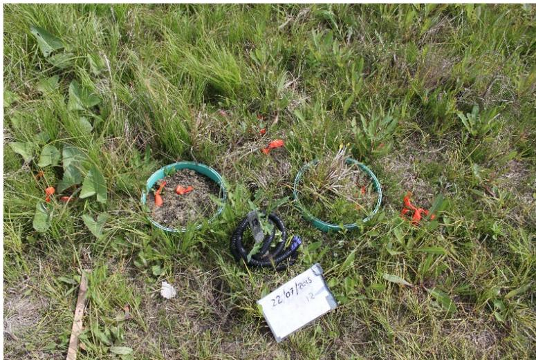
Figure 4 Soil collars for chamber measurements. One collar has roots excluded to assess soil respiration.
