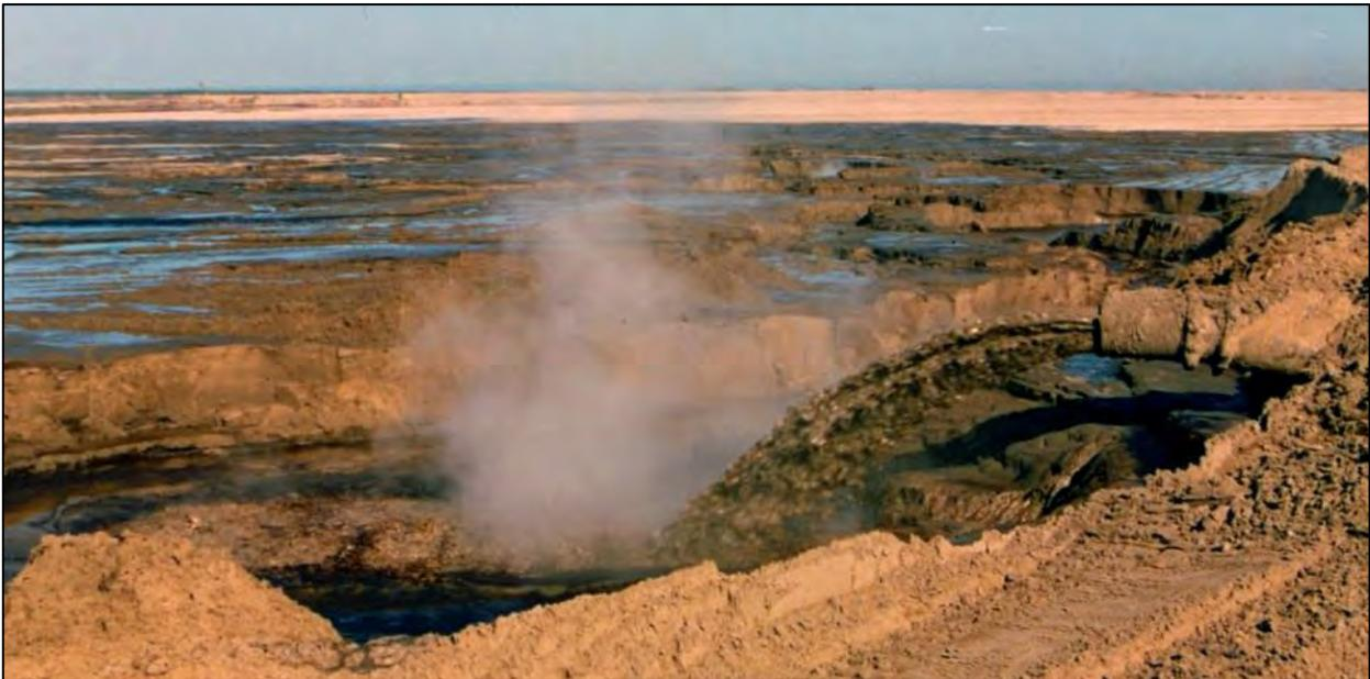
**Figure 2-1.** Extraction tailings slurry being discharged from a 24-inch-diameter pipeline for deposition onto a tailings sand beach.
