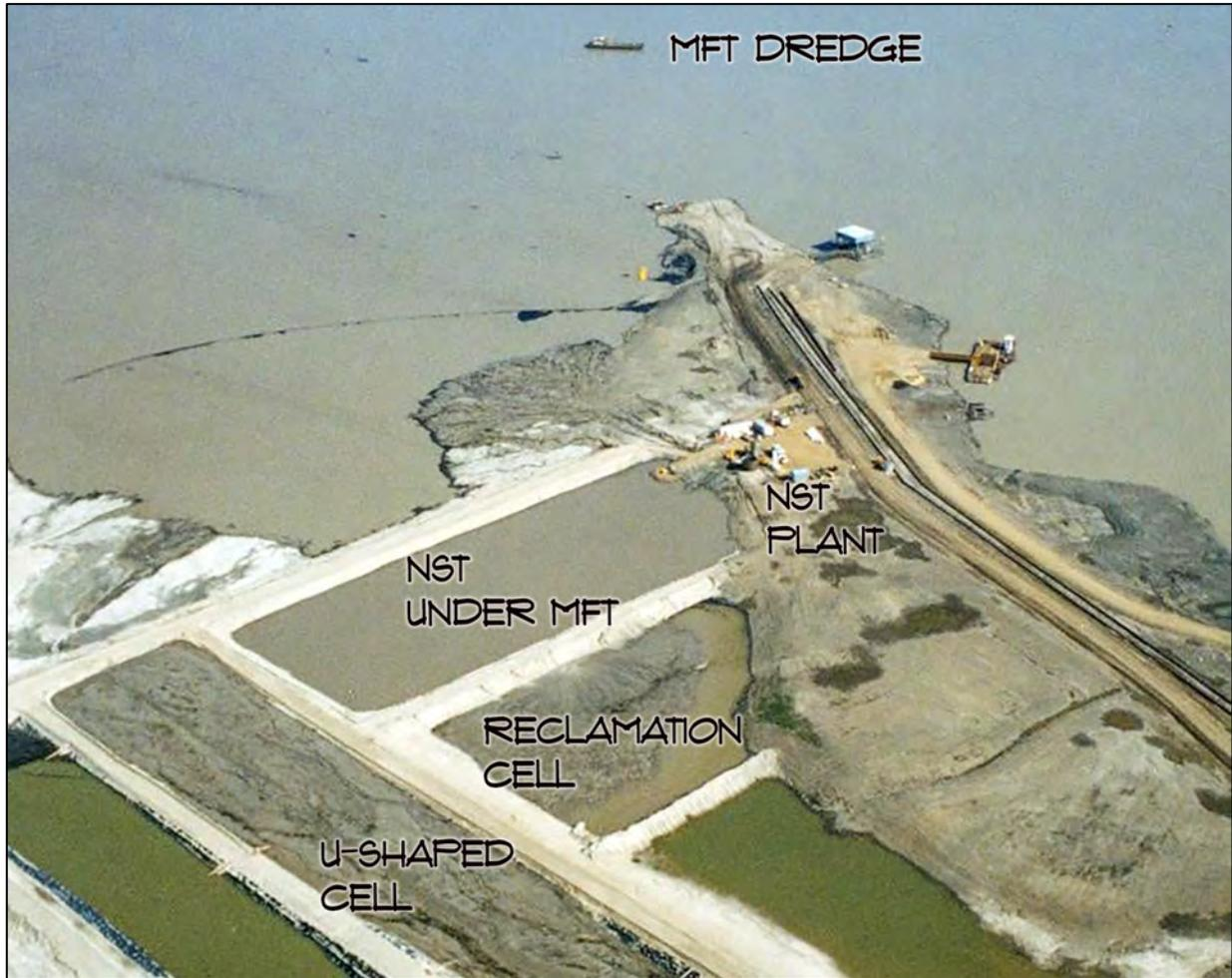
Figure 1-2. Syncrude 1995 NST Field Demonstration during deposition (NST U-shaped cell and reclamation cell).
