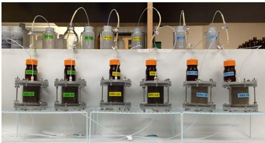
**Figure 4.2.** Photograph of experimental setup used for the column experiments.
