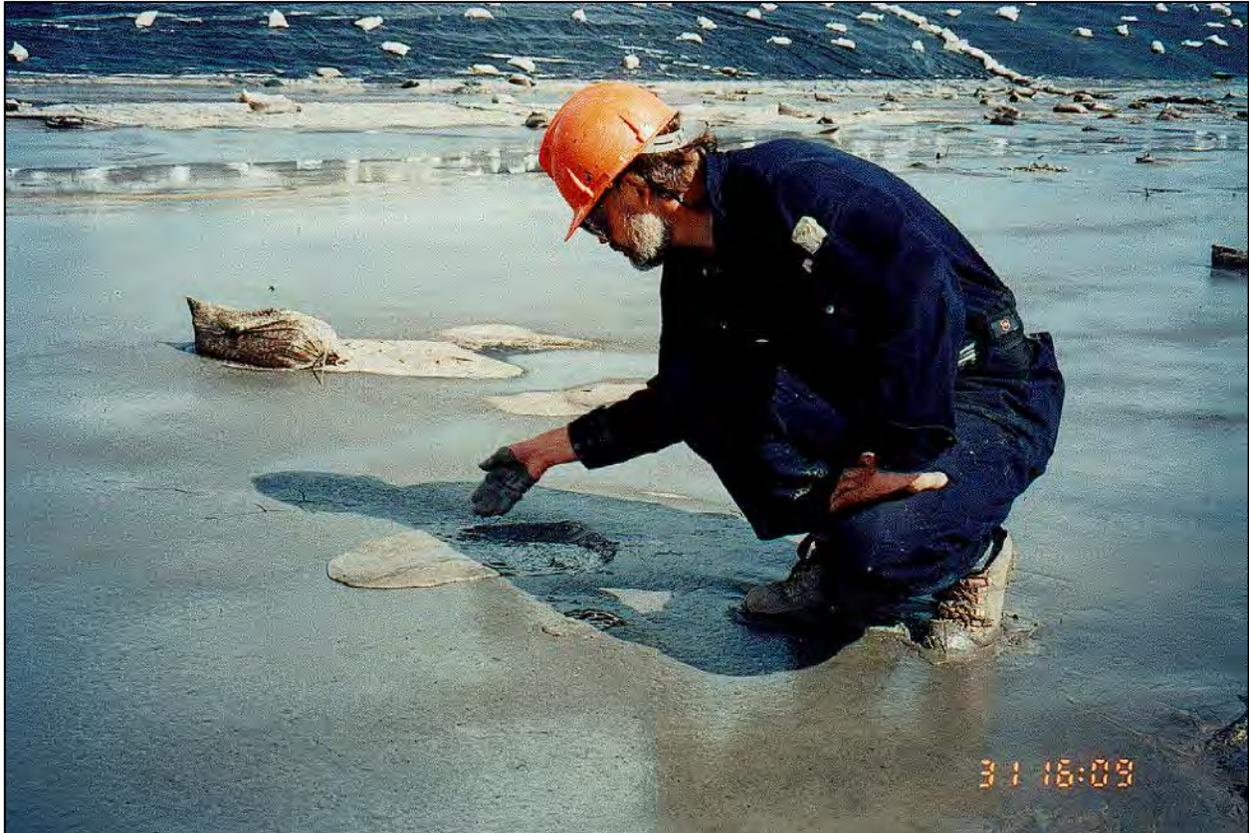
**Figure 2-2.** The initial few centimetre thick layer of freshly deposited CT in a test cell, about 70% solids content (NST Field Demonstration 1995).
