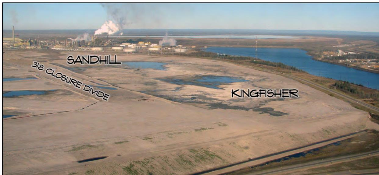
**Figure 4-13.** The 318 Closure Divide constructed on CT at EIP using hydraulic cell construction in 2007–2009.
