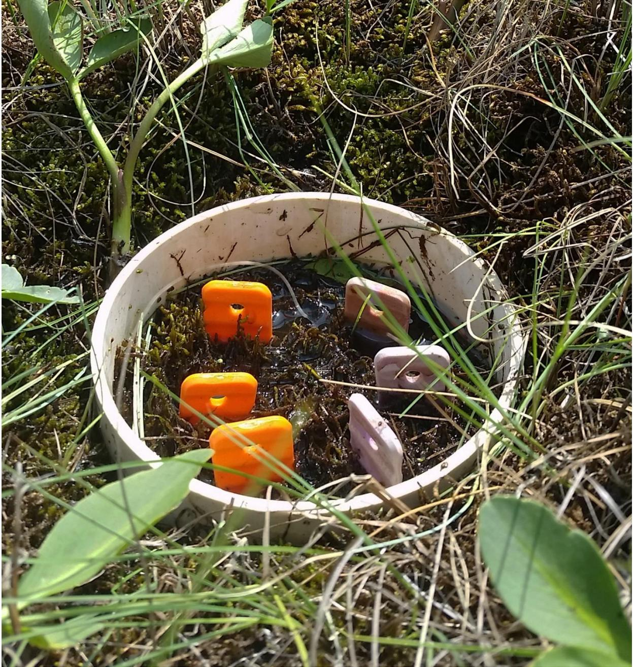
**Figure 5.4 Plant Root Simulator (PRS) probes inside a poly-vinyl-chloride cylinder**
