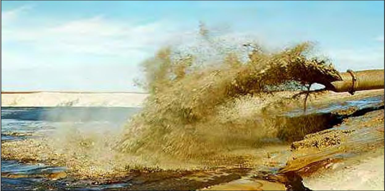
**Figure 3-7.** Tailings sand hydraulic beaching over CT using a spoon at the discharge – CT Prototype in 1998.
