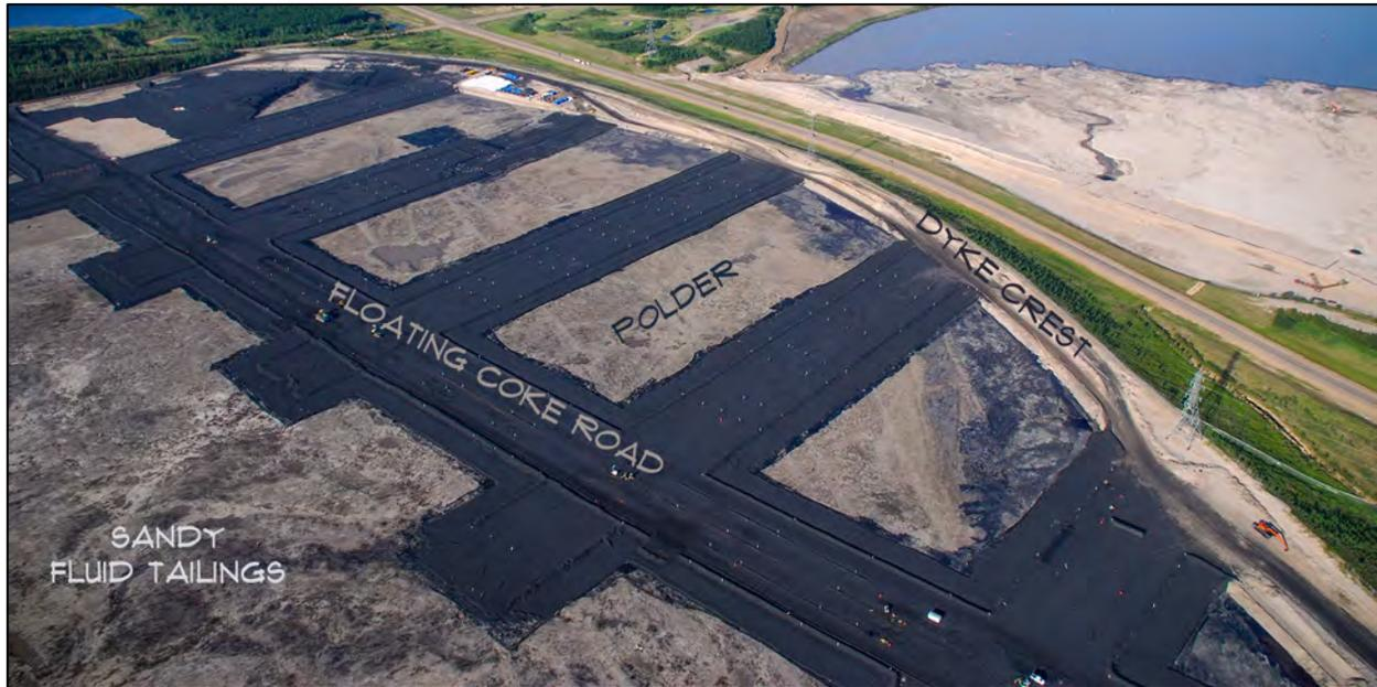
**Figure 3-4.** Mechanical placement of coke on off-spec CT at Suncor Pond 5 in 2010 (coke roads on strong geofabric).
