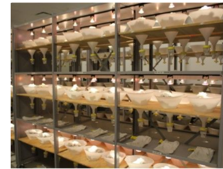
Figure 4. Berlese-Tullgren funnel apparatus in use.
