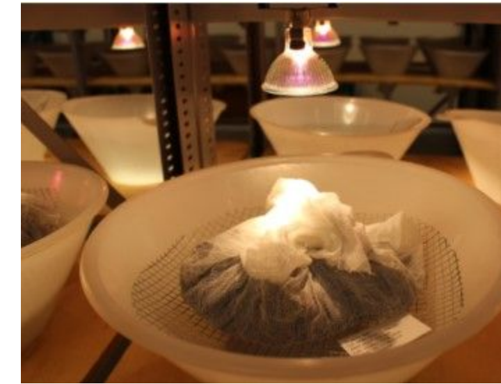
Figure 5. Top view of Berlese-Tullgren funnel apparatus in use.
