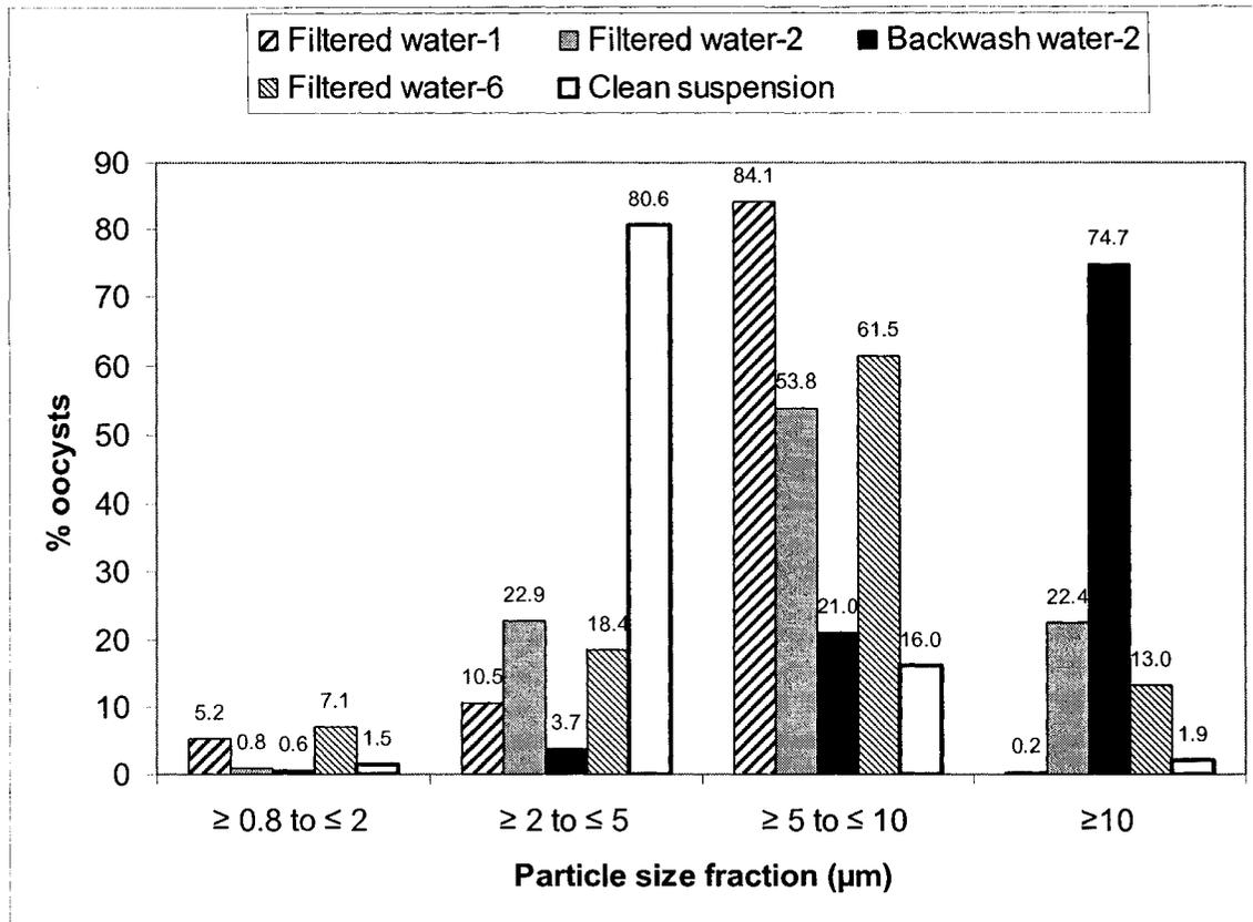
**Figure 4.6** Percent of total recovered oocysts retained on PCTE filters with different pore size
