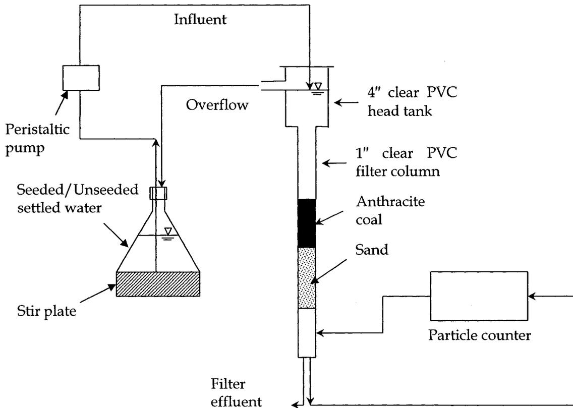
**Figure 3.2 Schematic diagram of the simulated filtration process**
