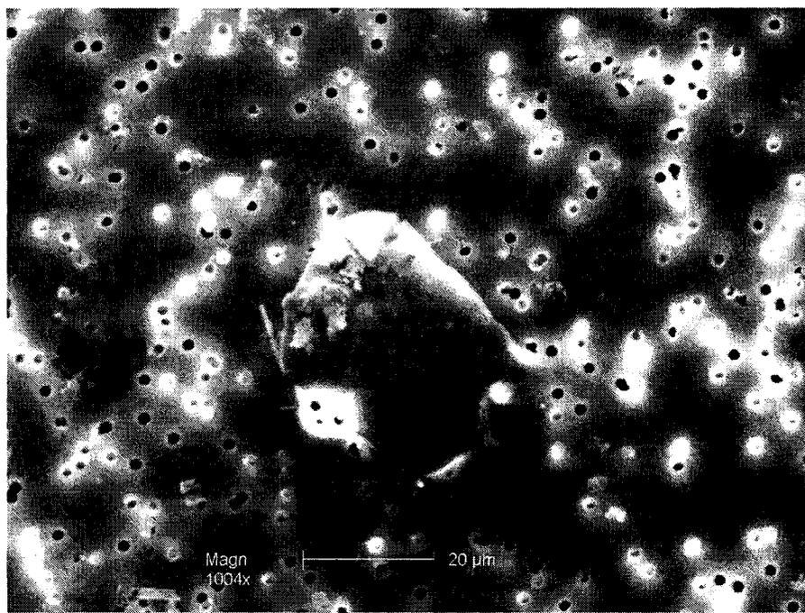
**Figure E.1 SEM micrograph showing a large particle captured on a 5 µm pore size PCTE filter from backwash water**
