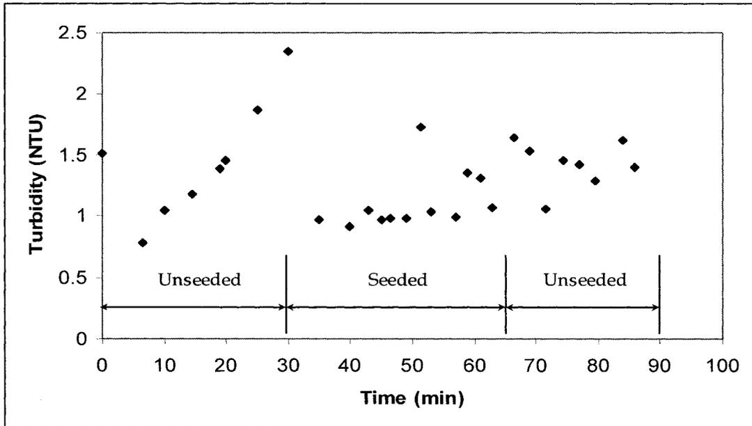
**Figure B.7 Turbidity of the filtered water as function of time for filtration run # 4**
