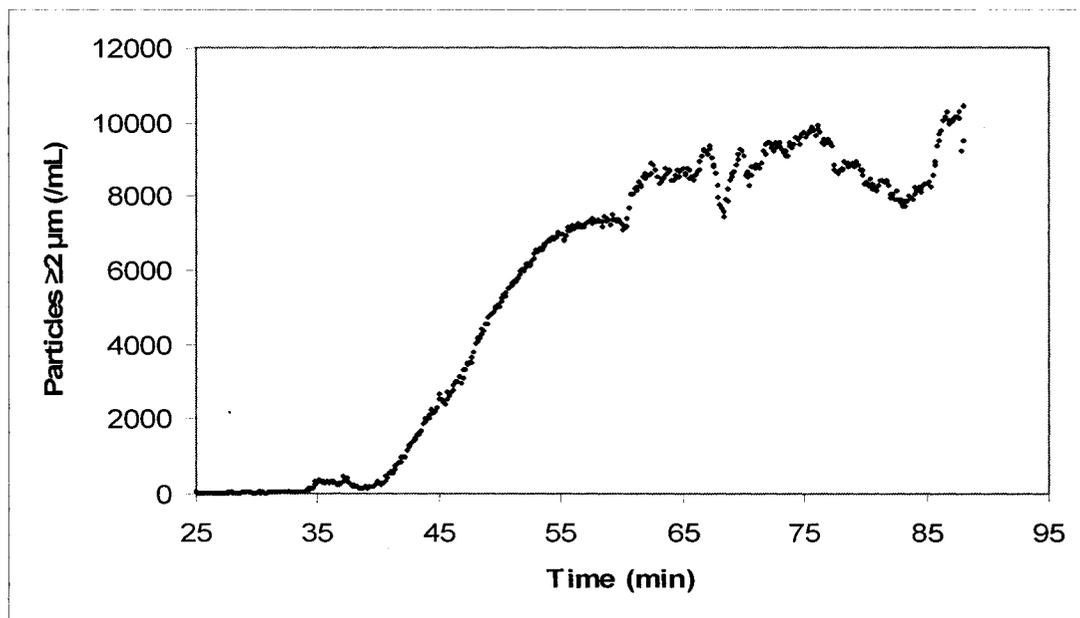
Figure B.10 Particle concentration of the filtered water as function of time for filtration run #5
