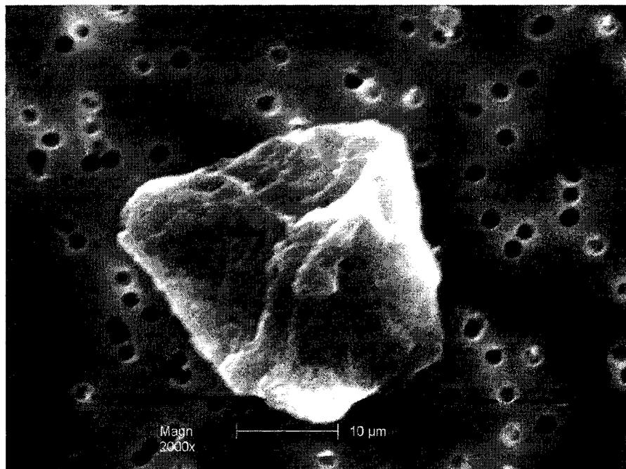
Figure 4.8 SEM micrograph showing large floc particle (approximately 30  $\mu\text{m}$ ) captured in a 5  $\mu\text{m}$  pore size PCTE filter
