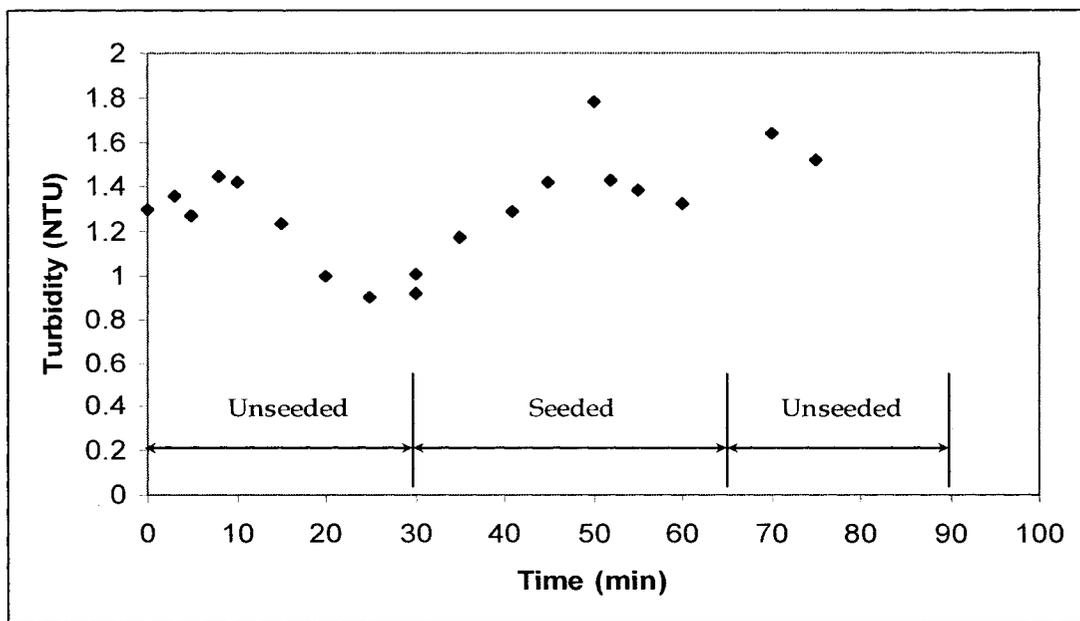
**Figure B.6 Turbidity of the filtered water as function of time for filtration run # 3**
