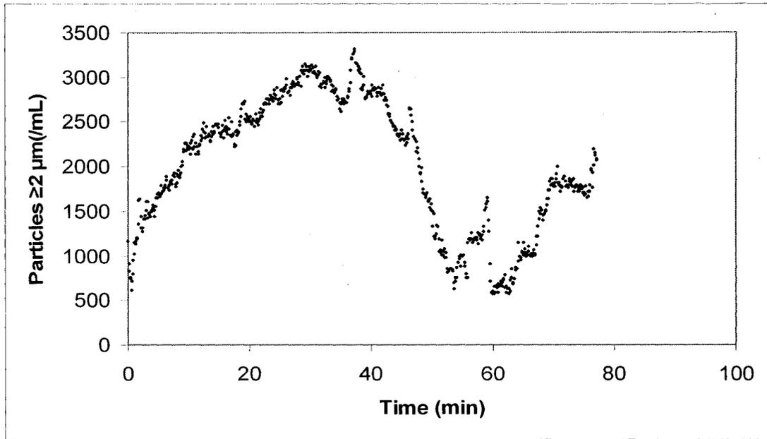
Figure B.12 Particle concentration of the filtered water as function of time for filtration run #6
