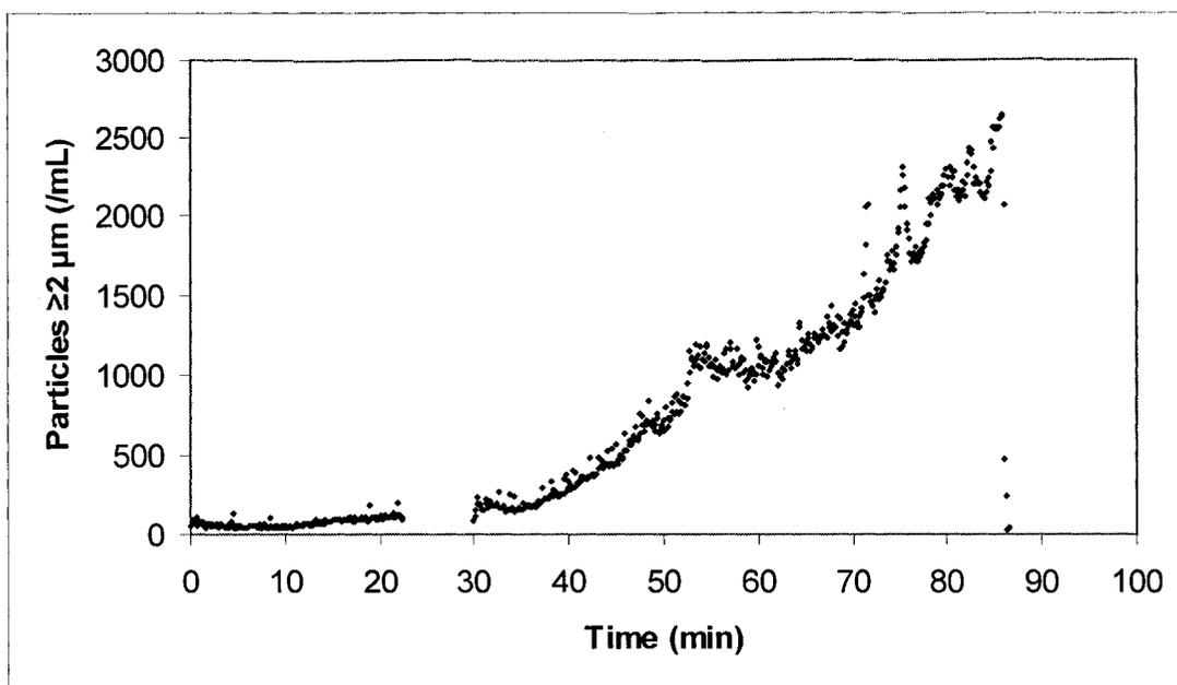
**Figure B.8** Particle concentration of the filtered water as function of time for filtration run #4
