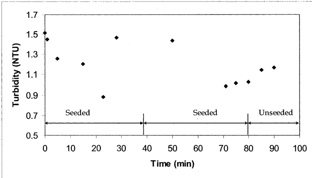
Figure B.4 Turbidity of the filtered water as function of time for filtration run # 2
