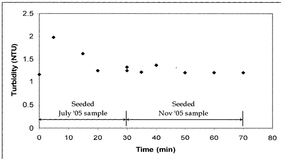
**Figure B.11** Turbidity of the filtered water as function of time for filtration run # 6
