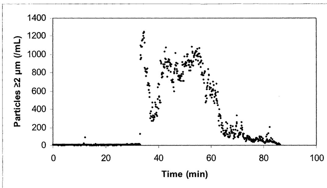
Figure B.3 Particle concentration of the filtered water as function of time for filtration run #1
