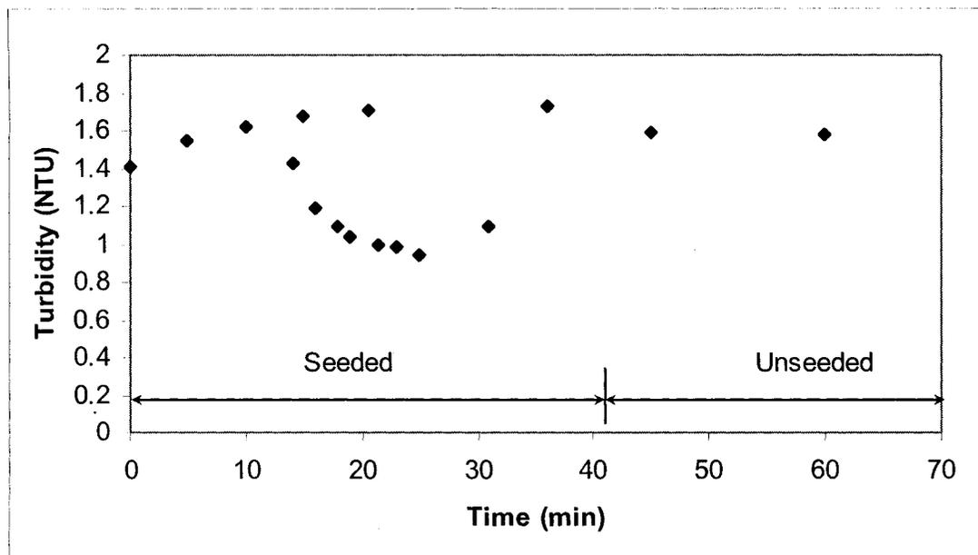
**Figure B.2** Turbidity of the filtered water as function of time for filtration run # 1
