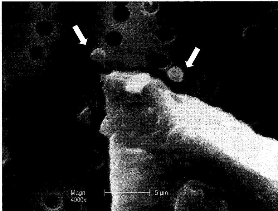
Figure 4.7 SEM micrograph of a large floc particle surrounded by *C. parvum* oocyst-like particles which might have been detached from the surface of the floc particle. The pore size of the PCTE filter was 5  $\mu\text{m}$ .
