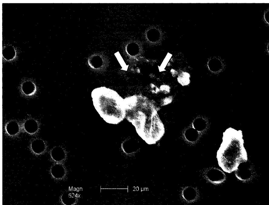
**Figure 4.9 SEM micrograph showing oocyst-like particles attached to other particles captured on the surface of a 10 µm pore size PCTE filter**
