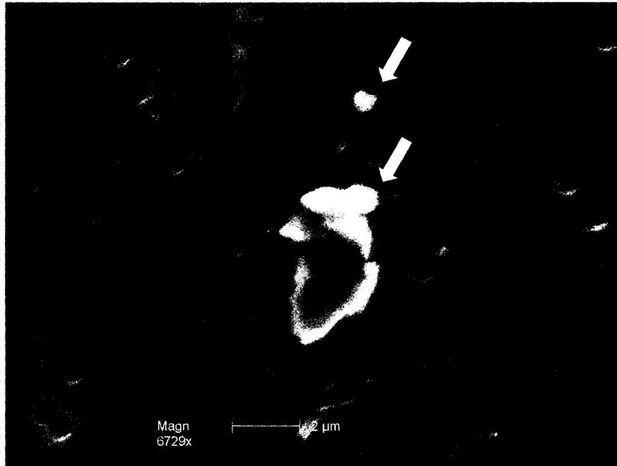
**Figure E.4** SEM micrograph of a flocculent particle with *C. parvum* oocysts-like particle attached to the surface of the flocculent particle. The pore size of the PCTE filter was 5 μm.
