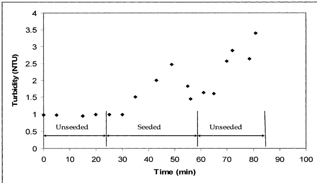
Figure B.9 Turbidity of the filtered water as function of time for filtration run # 5
