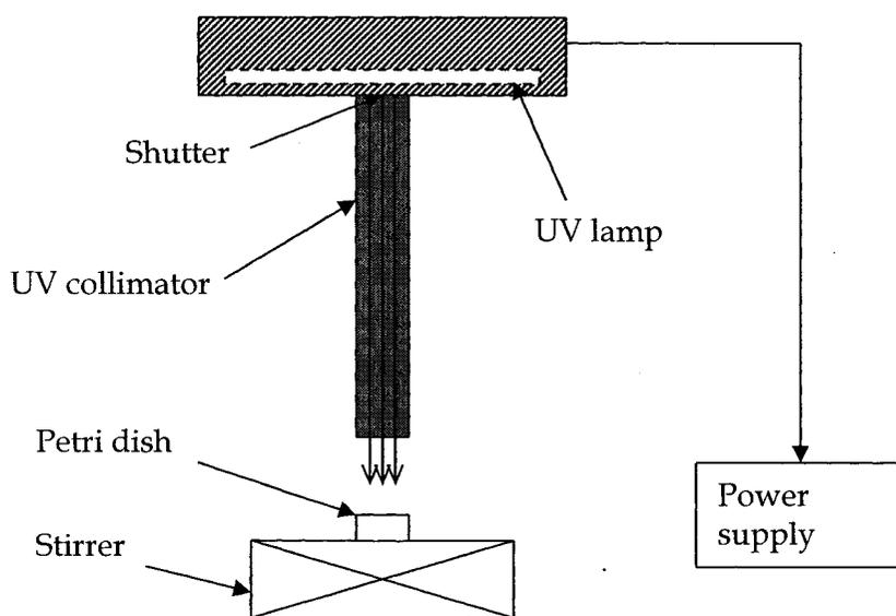
Figure 2.4 Schematic diagram of a collimated beam apparatus
