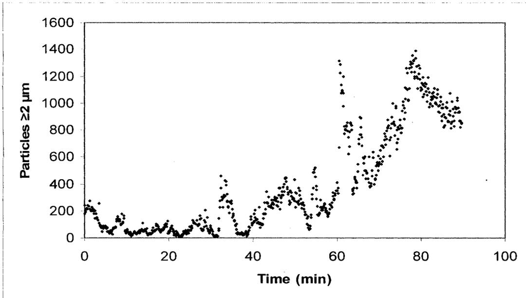
Figure B.5 Particle concentration of the filtered water as function of time for filtration run #2
