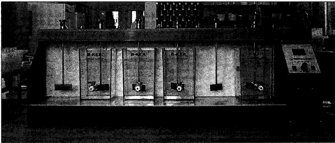
**Figure 3.1** Jar testing apparatus used for simulation of coagulation, flocculation and settling
