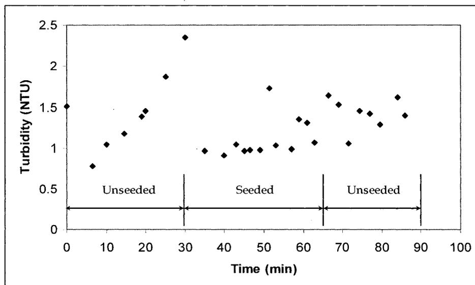
Figure 4.3 Turbidity of the filtered water as function of time for filtration run no.4. Time zero corresponds to the start of the filtration run.
