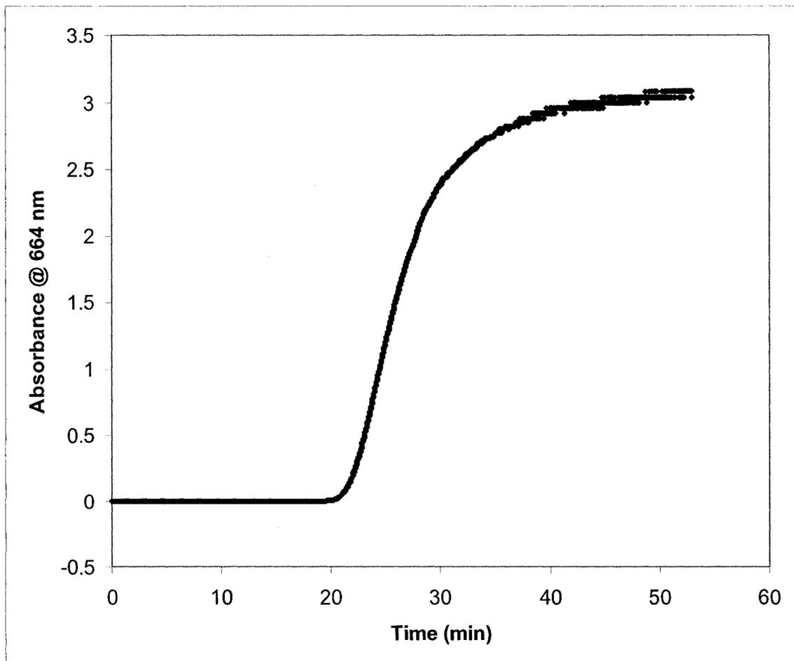
Figure B-1 Tracer test on filter column using methylene blue
