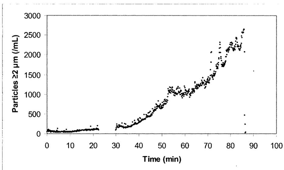
Figure 4.4 Particle concentration of the filtered water as function of time for filtration run no. 4. Time zero corresponds to the start of the filtration run.
