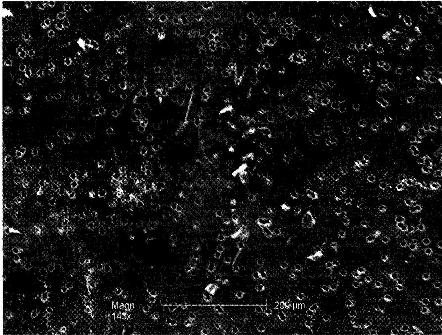
**Figure E.2** SEM micrograph showing particles captured on a 10 µm pore size PCTE filter from backwash water
