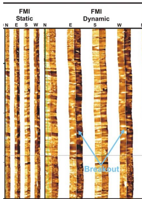
Figure 8. Borehole breakout observed on Formation Micro Imager (FMI) log (Bell, 1996)
