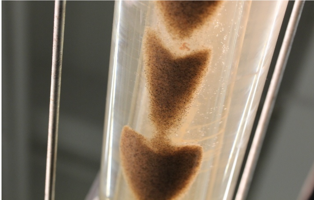
Figure 6 - 15. Dunes/Saltation Pattern at Velocity of 0.33 m/s - Water Flow - Mean Particle Diameter: 350 Microns - View from the Bottom of the Pipe.
