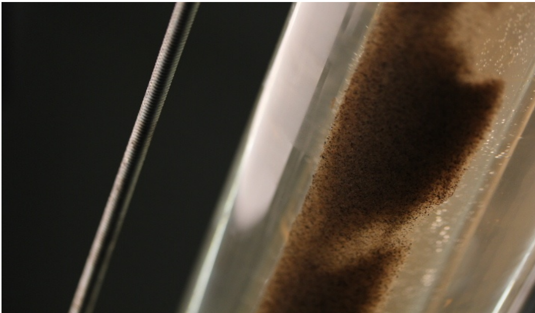
Figure 6 - 12. Dunes/Saltation Pattern Starts Forming at Velocity of 0.26 m/s - Water Flow - Mean Particle Diameter: 350 Microns - View from the Bottom of the Pipe.
