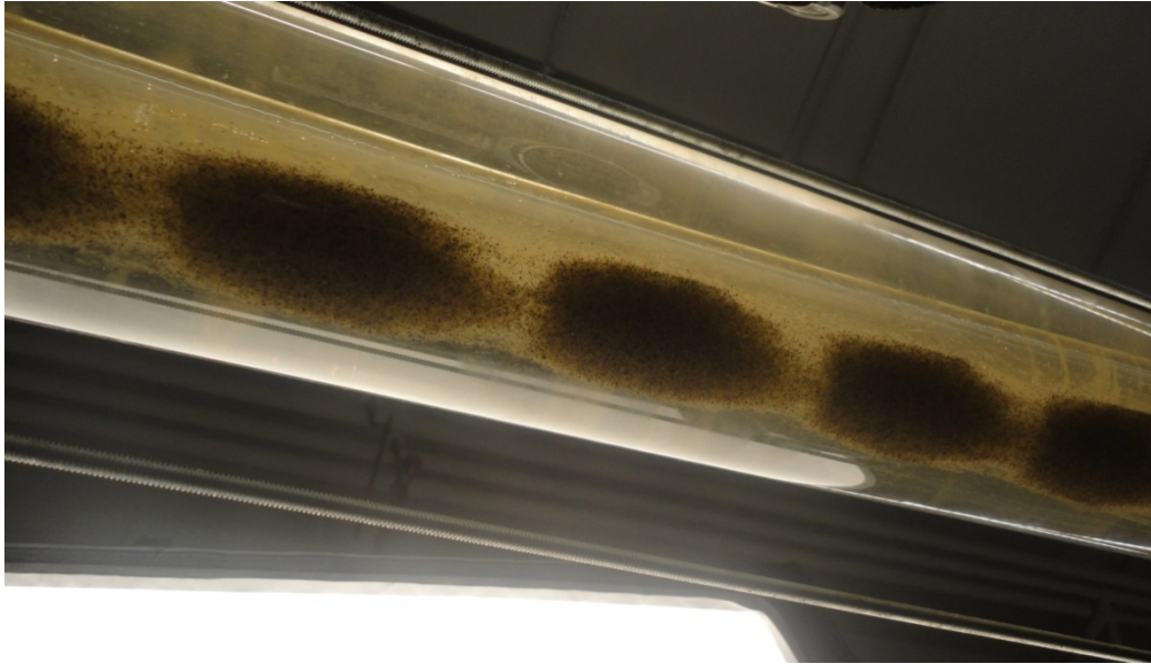
Figure 6 - 21. Dunes/Saltation Pattern at Velocity of 0.96 m/s - 0.07% V/V PHPA Solution - View from the Bottom of the Pipe - Mean Particle: 350 Microns.
