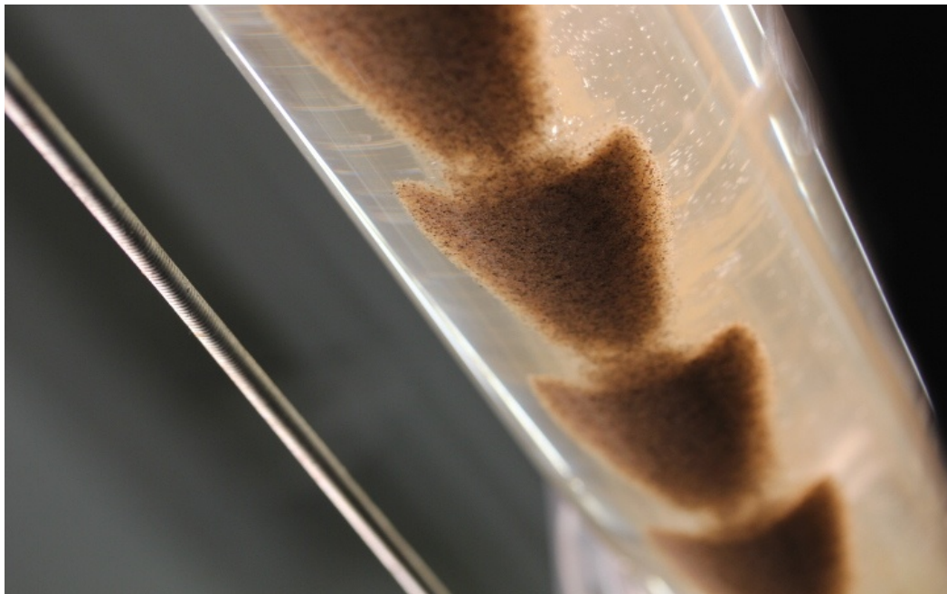
Figure 6 - 14. Dunes/Saltation Pattern at Velocity of 0.28 m/s - Water Flow - Mean Particle Diameter: 350 Microns - View from the Bottom of the Pipe.
