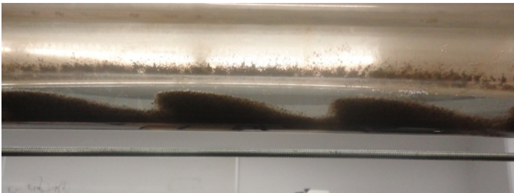
Figure 6 - 20. Dunes/Saltation Pattern at Velocity of 0.96 m/s - 0.07% V/V PHPA Solution - View from the Side of the Pipe - Mean Particle Diameter: 350 Microns.
