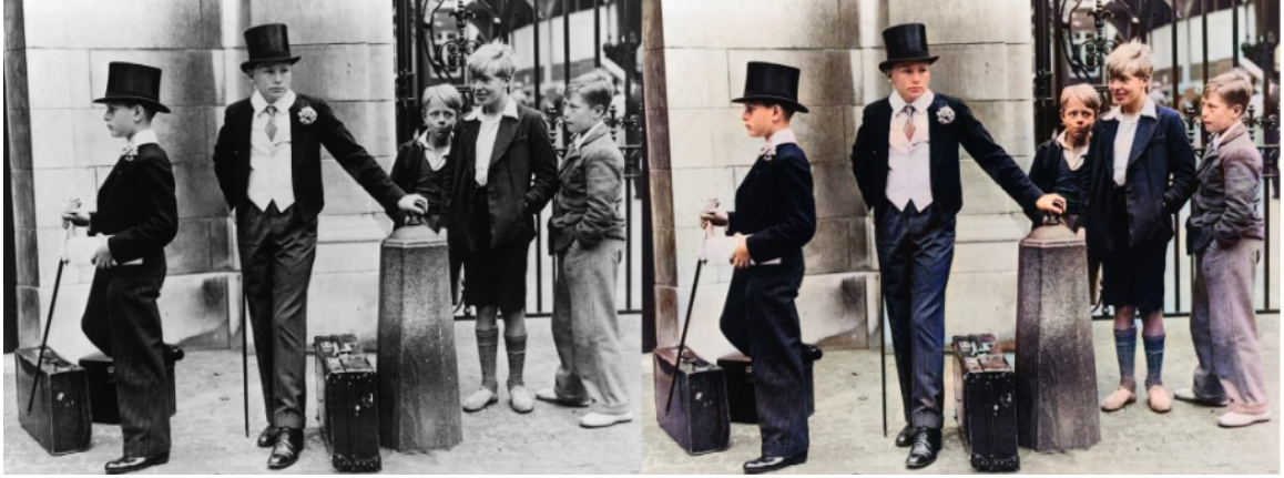
Figure 1.2: An image colorization example by Deoldify [10], where the left one is the input and the method will automatically output a colorized version on the right.
