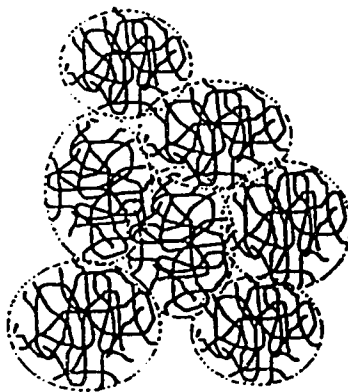
Fig. 2.2-12 - Space-filling clusters. From Brinker et al. [40]
