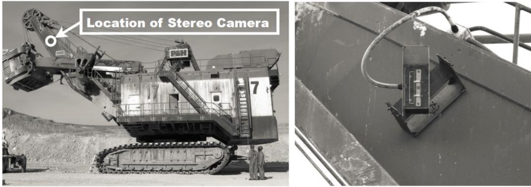
Figure 2.9 Location of the stereo camera and a close-up photo of the camera in its protective mount on the right (Brothwick, 2009)
