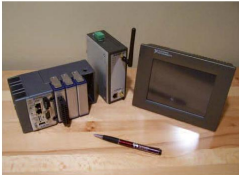
Figure 5.11 Data acquisition, wireless transmitter and touch screen processor (Joseph & Chamanara, 2012)
