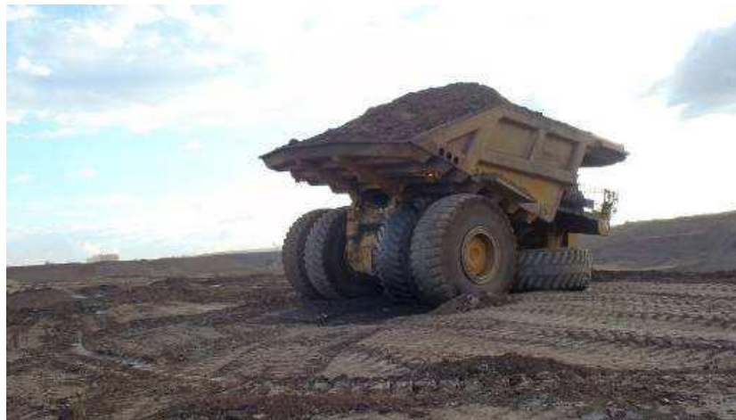
Figure 2.28 RHF spindle failure on a 797B truck (Rear view) (Finning, 2010)
