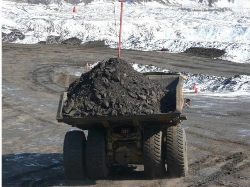
Figure 1.1 Caterpillar 797B haul truck under an unbalanced load
