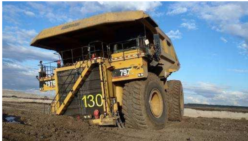
Figure 2.27 RHF spindle failure on a 797B (Front view) (Finning, 2010)
