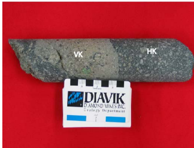
Figure 2-3. Sample of drill core from A154S. Autolithic HK surrounded by a mud-rich VK.
