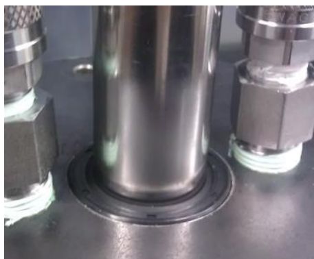
Figure 3-9 (b): The Seal to isolate the contents inside from the outer atmosphere
