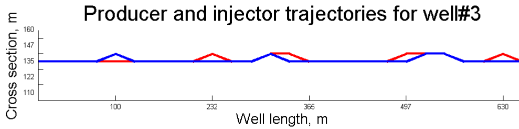
(b) Top view for undulate trajectory method (blue: producer, red: injector)
