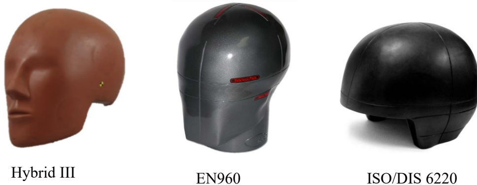
Figure 2.9. Commercially available headforms commonly used in head injury research and helmet tests. Images of headforms based on EN960 and ISO/DIS 6220 standards were from cadexinc.com, and used with permission.
