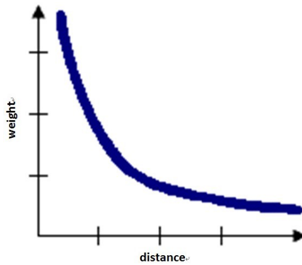
Figure 4.4: The relationship between the spatial weight and the distance under inverse distance model (with \delta = 1.0 )
