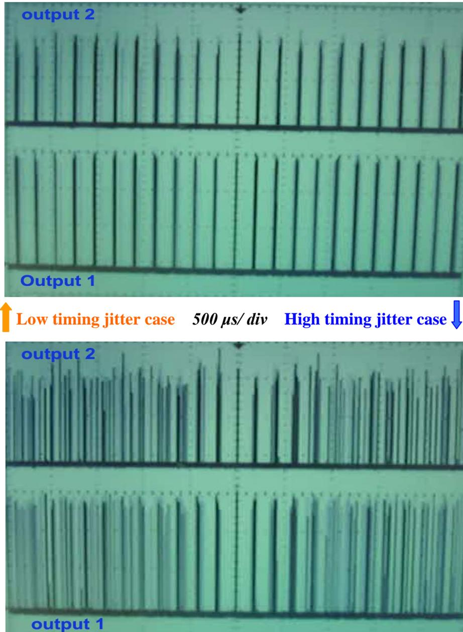
Figure 8.4: Grabbed pictures from the video recording the pulse trains. The upper traces show the picture when the laser sticking to pulse repetition rate and the lower traces show hte cases when the laser was in a high timing jitter state. The pulse trains were recorded at an absorbed pump power of 0.65 W with a pulse repetition rate of  $\sim 5\text{kHz}$ .
