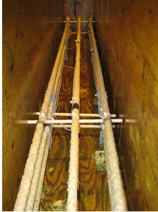
Figure C-4: Rebar cage positioned in the 600 mm deep formwork (specimen B6H). The No. 3 transverse support bars seen in the center of the photograph are located at mid-span. Similar support bars were provided at both ends.
