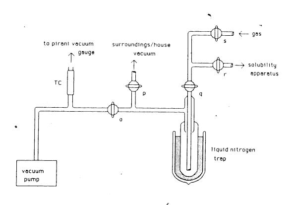
Fig. 4.4. Schematic diagram of the vacuum assembly: TC, thermocouple gauge; o, p, q, r, s, Kontes teflon valves.
