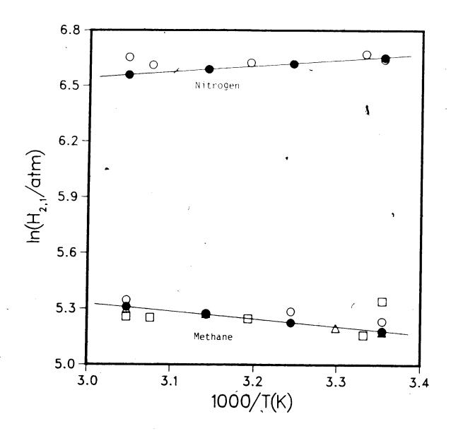
Fig. 5.1. Henry's constants for nitrogen and methane in hexadecane.
