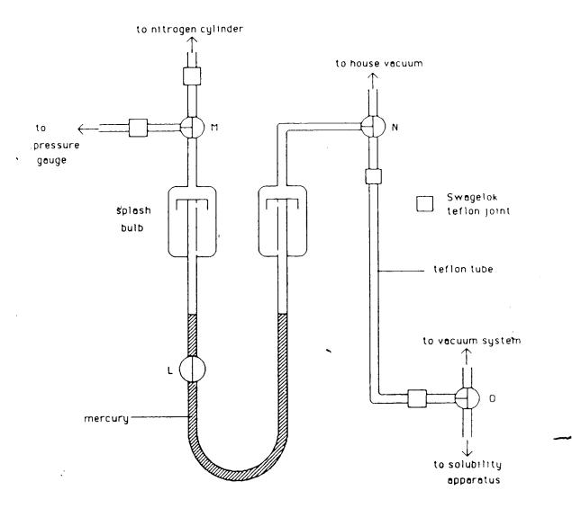
Fig. 4.2. Schematic diagram of pressure balance: M, N, O, three-way teflon valves; L, two-way teflon valve.
