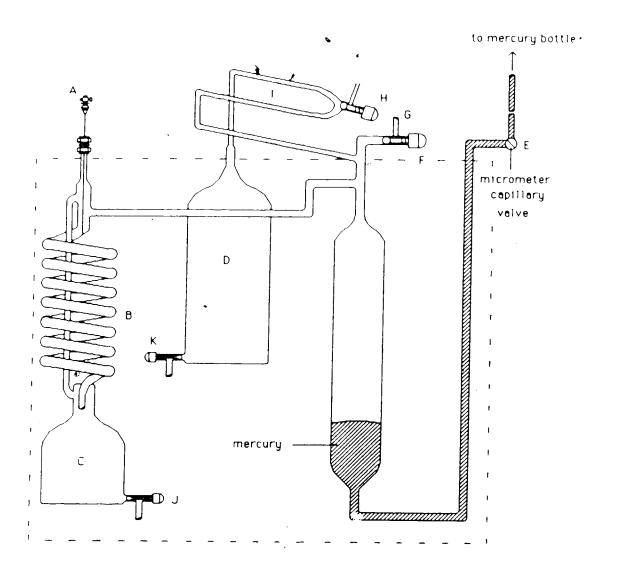
Fig. 4.1. Schematic diagram of the isobaric equilibrium apparatus for determining gas-liquid solubilities: A, Mininert teflon valve; B, spiral; C, receiver; D, buffer; I, U-tube; E, micrometer capillary valve; J, K, H, F, Kontes teflon valves; G, for connection to vacuum assembly/pressure balance apparatus. The dotted line represents a water-filled thermostatted bath.
