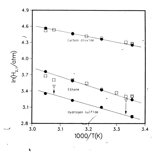
Fig. 5.2. Henry's constants for carbon dioxide, ethane, and hydrogen sulfide in hexadecane. Carbon dioxide: ●, this work; ○, GC; □, Ref. 69, 89. Ethane: ●, this work; ○, GC; □, Ref. 67, 69, 91. Hydrogen sulfide: ●, GC; ▽, Ref. 70,89.
