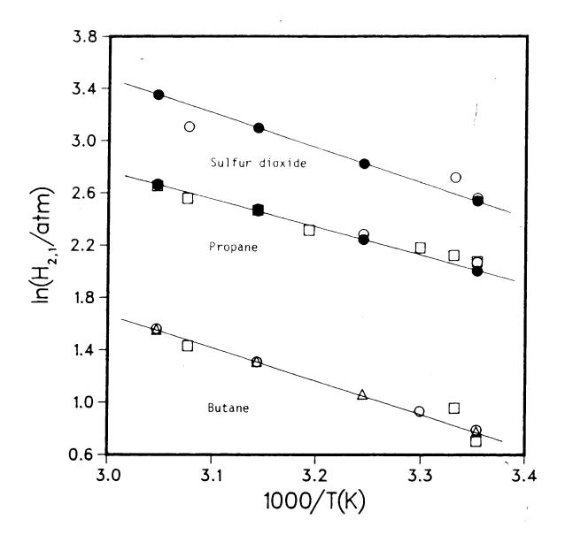
Fig. 5.3. Henry's constants for sulfur dioxide, propane, and butane in hexadecane. Sulfur dioxide: ♠, this work; ♠, Ref. 70, 89. Propane: ♠, this work; ♠, GC; ♠, Ref. 67, 69, 92. Butane: ♠, GC; ♠, Ref. 67; ♠, Ref. 70, 92.
