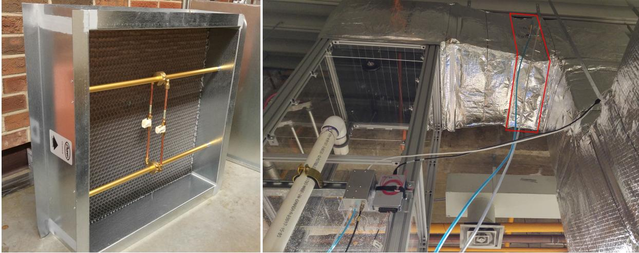
**Figure 4.13** – Dwyer STRA averaging pitot tube installed in experimental model
