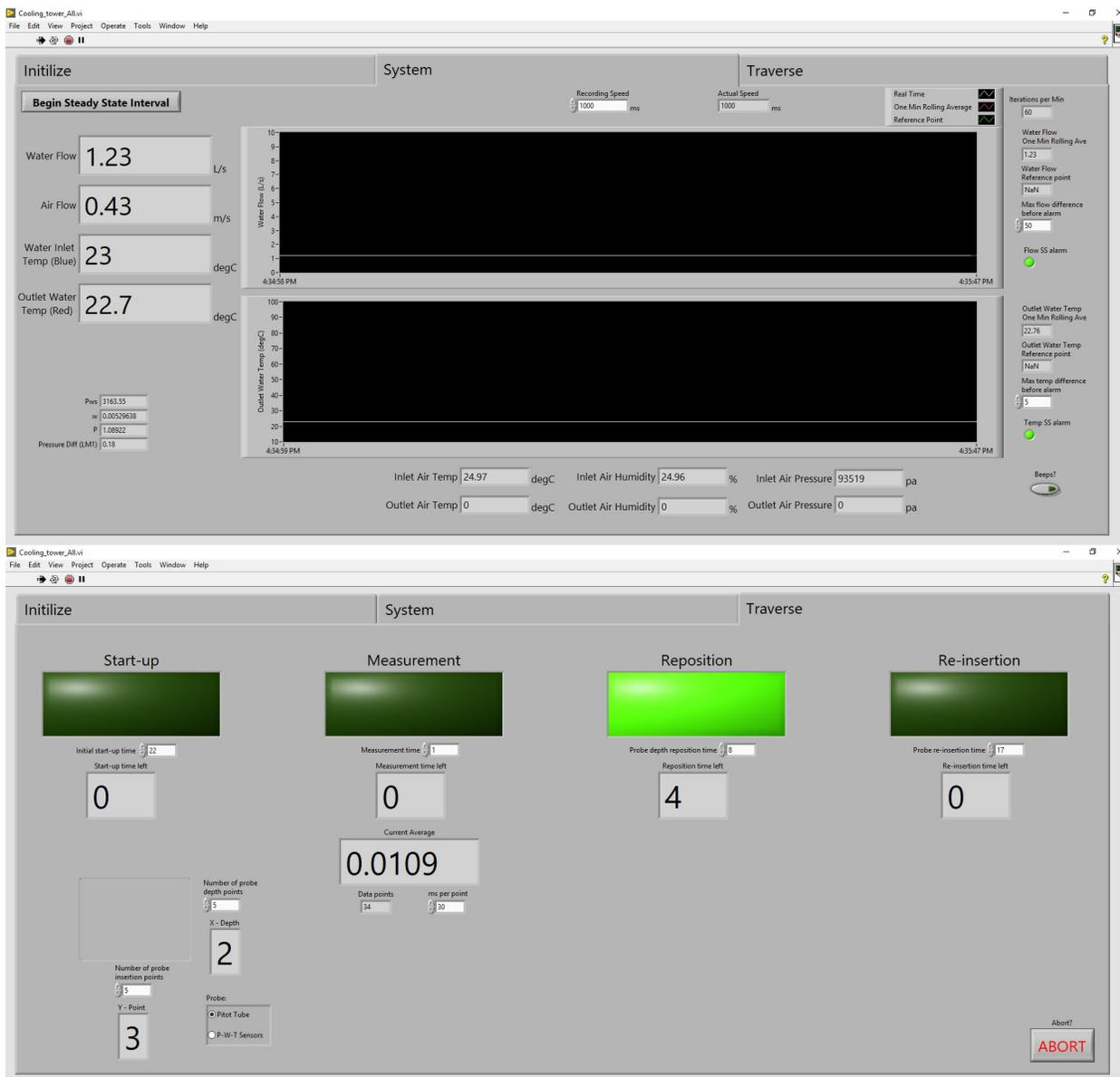
Figure 3.7 – LabView GUI for collection of sensor data
