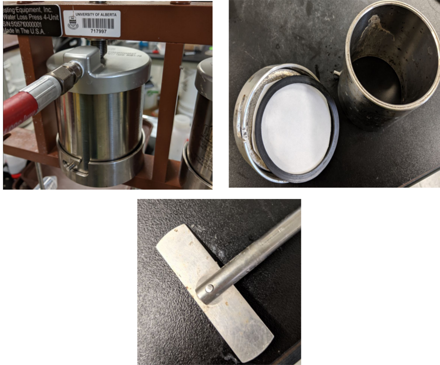
Figure 4.2: The impeller and the air-pressurized filtration unit used for mixing and dewatering of MFT.
