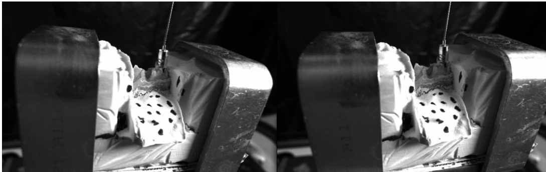
Figure B-1: Two video frames demonstrating self-alignment of potted samples in the experimental apparatus. Left: alignment at the outset of loading; Right: alignment after 50N transition.
