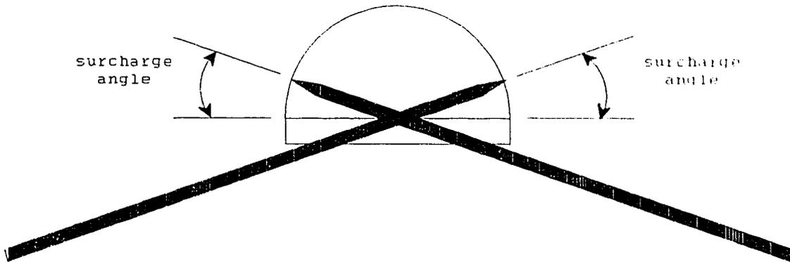
Figure 6.2 Surcharge angle measuring device
