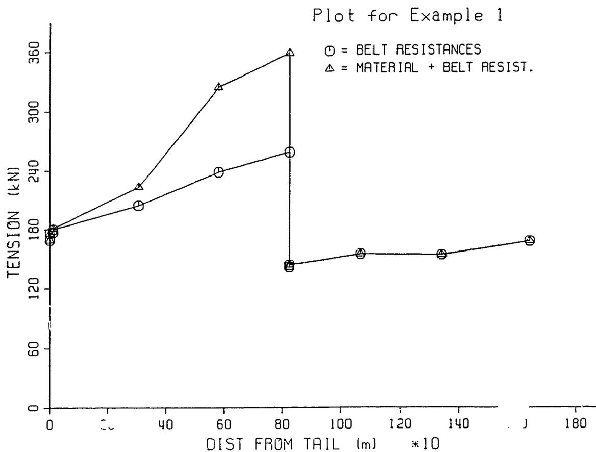
Figure A.2 Graphical form of belt tensions for Example #1
