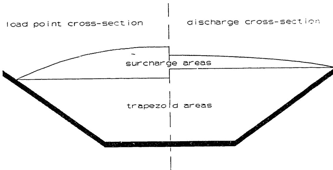
Figure 6.5 Cross-section comparisons
