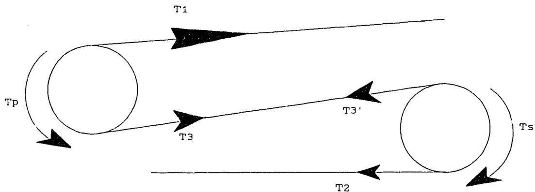
Figure 4.2 Tensions around dual drive pulleys
