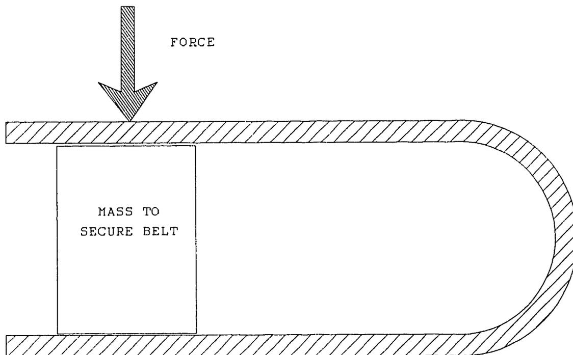
Figure 5.1 Sketch of belt bending test
