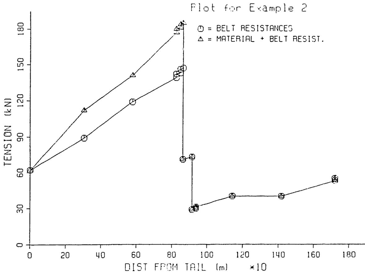
Figure A.4 Graphical form of belt tensions for Example #2
