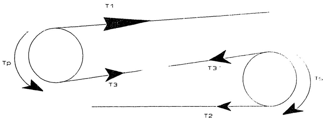
Figure 3.4 Tensions around a dual pulley drive
