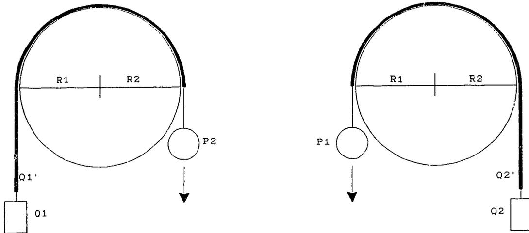
Figure 5.5 Sketch of forces around pulley
