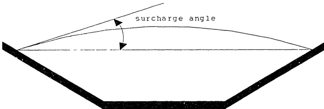
Figure 6.1 Diagram illustrating surcharge angle
