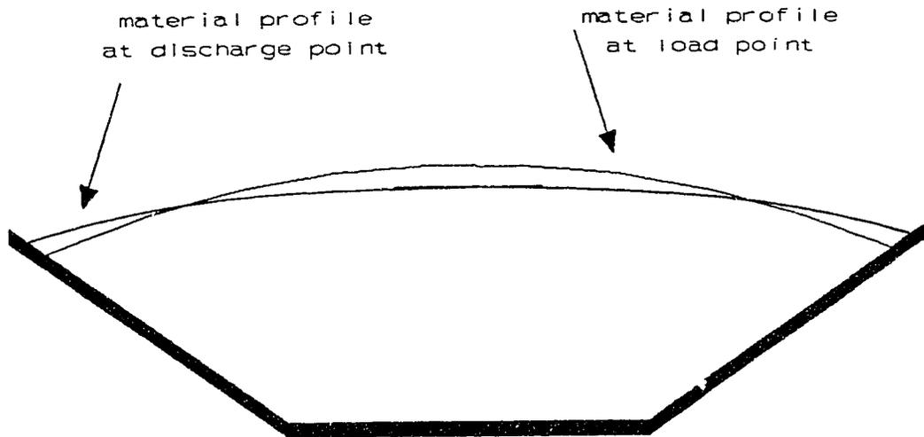
Figure 6.4 Oil sand profile at load point and discharge point
