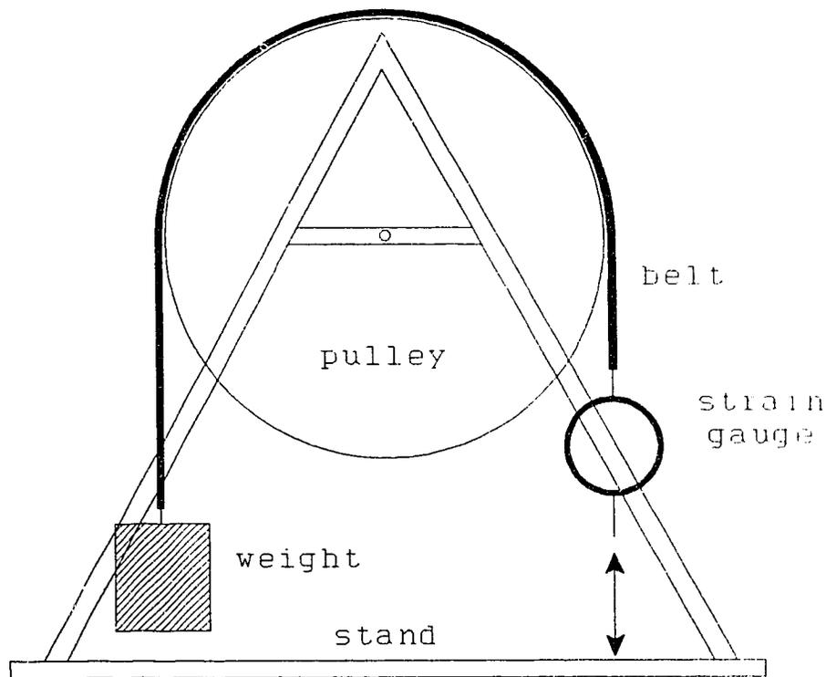
Figure 5.4 Belt flexure apparatus
