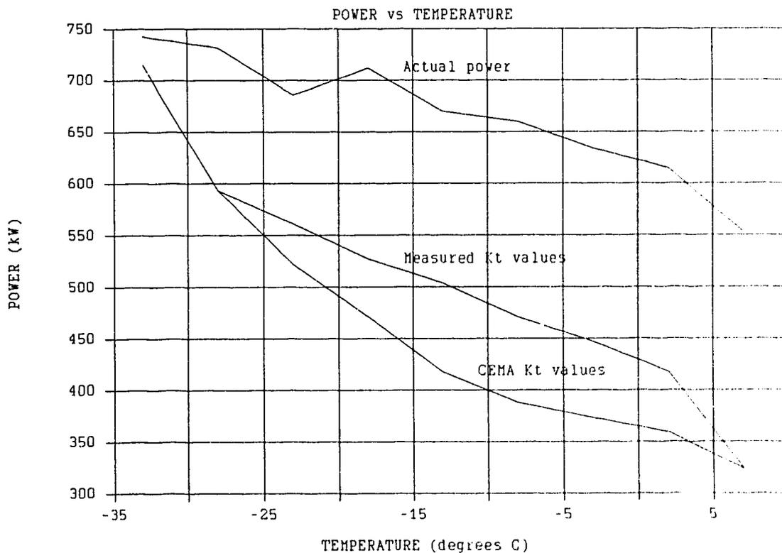
Figure 5.3 Plot of theoretical and actual power requirements
