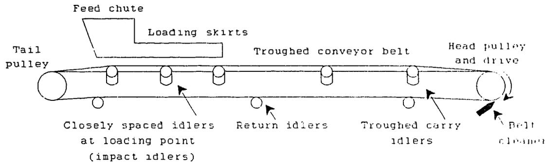
Figure 4.1 Major components of conveyor and material resistance to movement
