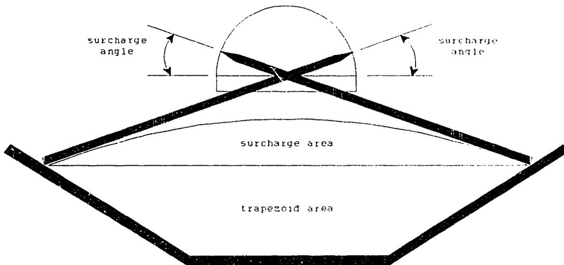
Figure 6.3 Positioning of measuring device on oil sand
