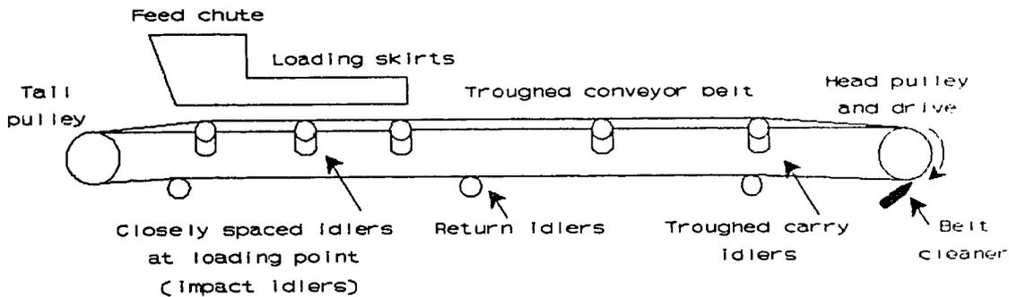
Figure 2.1 Idealized troughed belt conveyor
