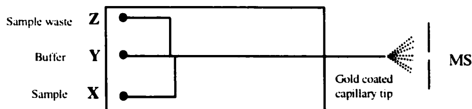
Figure 2-4. The microchip layout for ESMS from a PCRD-1 chip (detailed layout information in Figure 2-5). The capillary tip was 3 cm long. Sample was in reservoir X and sample waste was Z. Injection: X (-3.5 kV) to Z (ground), gold capillary tip (ground). Separation: Y (-3.5 kV) to capillary tip (3.2 kV), with push back voltage at X and Z (-2 kV). The power supply relay connection network is shown in Figure 2-7.
