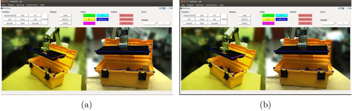
Figure 5.13: (a) The user selects a line and two points. (b) He/she then clicks on the L-L button to get the resulting line-to-line task. Since only one line was created beforehand, the second line was added automatically when the user specified the task.
