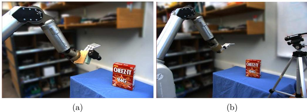
Figure 3.3: (a) Eye-in-hand and (b) eye-to-hand camera configurations.
