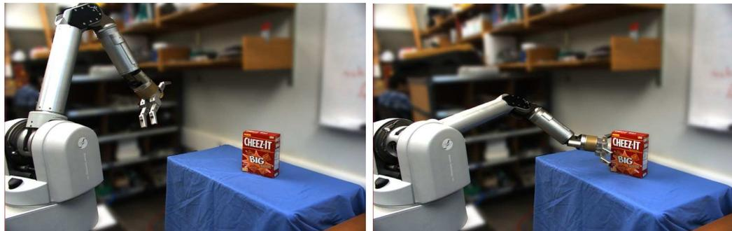
Figure 3.2: Visual servoing moves the end-effector to a desired location in the workspace to get close to an object in order to grasp it.
