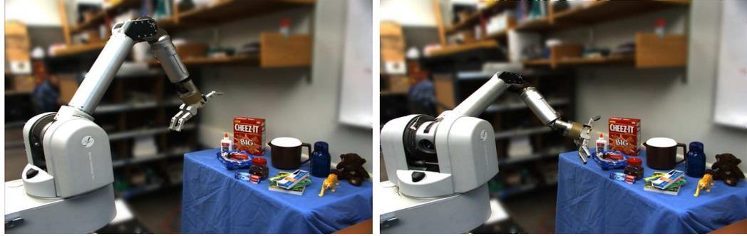
Figure 2.2: Robotics in an uncontrolled environment. The robot needs to grasp objects from a cluttered table. Grasping any of the objects requires a combination of coarse movements and fine manipulation.
