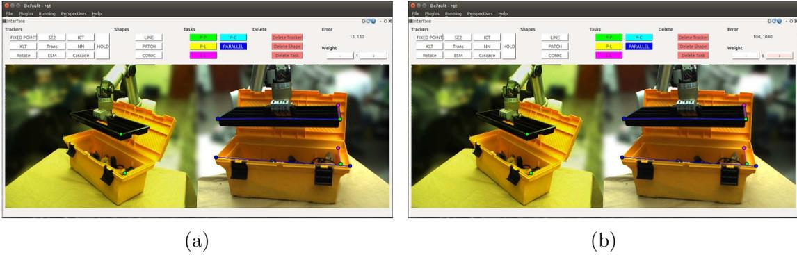
Figure 5.18: When in layer view the user can adjust the weight of the task being viewed. (a) The task error is displayed to the right in the interface. (b) By pressing the '+' button the user changes the scale to 8.
