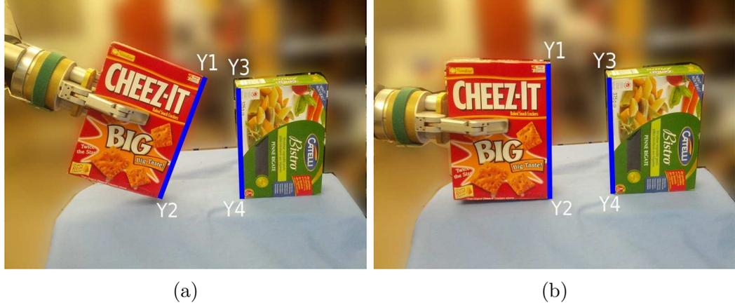
Figure 4.5: A parallel lines task is specified (a) and completed (b). Each  $y_i$  is a 2D point.
