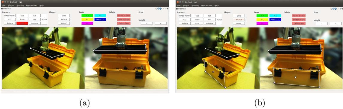
Figure 5.6: The user clicks on the ESM button (a) and then clicks on four points in the image to initialize a new ESM patch tracker (b).
