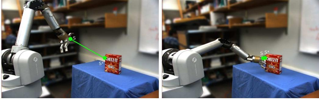
Figure 3.5: Image based visual servoing by minimizing the error between a 2D point feature on the robot,  $s$ , and a goal point feature,  $s^*$ , on the object.
