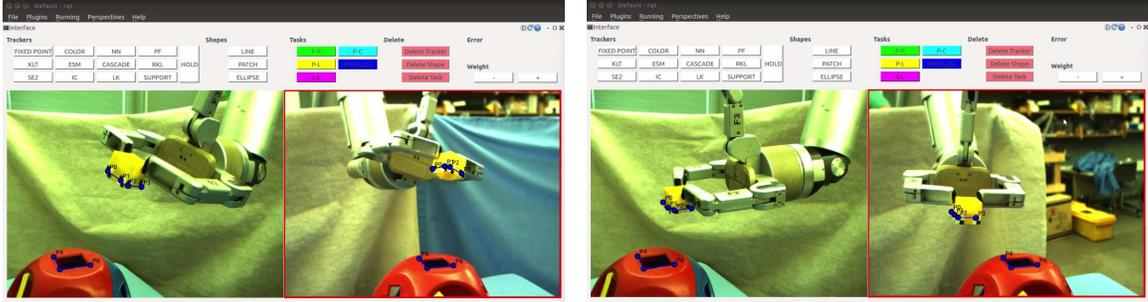
Figure B.7: We align the orientation of the cube with the square opening by specifying two parallel lines tasks. At the end of the alignment some of the trackers are about to get lost and we need to change the camera view.
