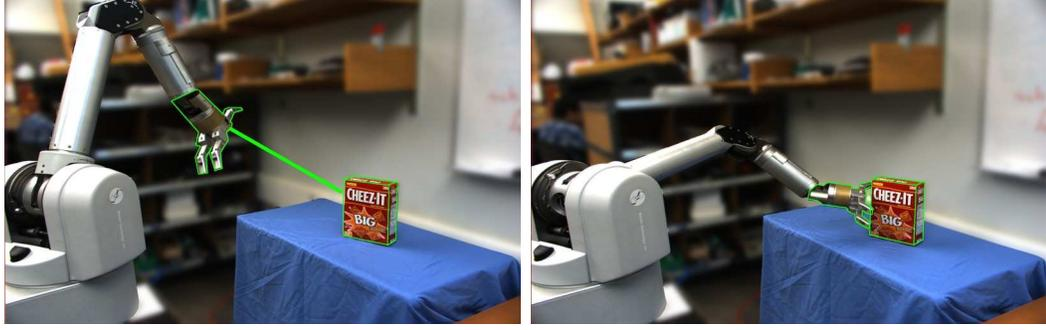
Figure 3.4: Position based visual servoing moves the robot based on knowledge of the robot end-effector pose and the object pose.
