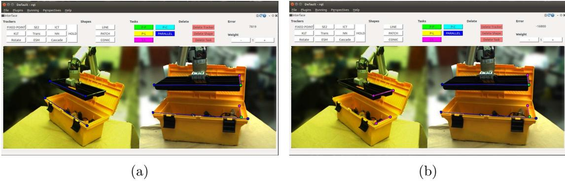
Figure 5.17: By pressing the L key the user can enter layer view in one of the camera views. It allows the user to shuffle through and see each task individually. Any other points, shapes or tasks are invisible. (a) The user sees only the parallel lines task in the left image view. (b) The user sees only the line-to-line task in the left image view.
