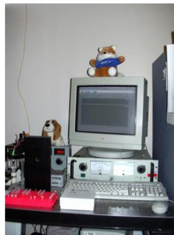
**Figure 2.2. Diagram and photographs of the laboratory-built capillary electrophoresis laser-induced fluorescence (CE-LIF) instrument used in this research**
