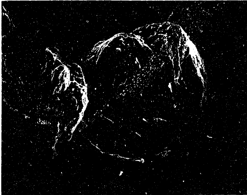
PLATE 3 SEM Micrograph of a Cross Section of Raw Fluid Petroleum Coke, (x200).
