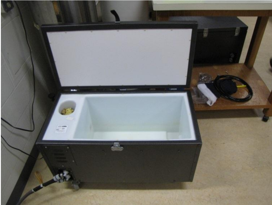
Plate C3. The reservoir and pump system used to circulate water.
