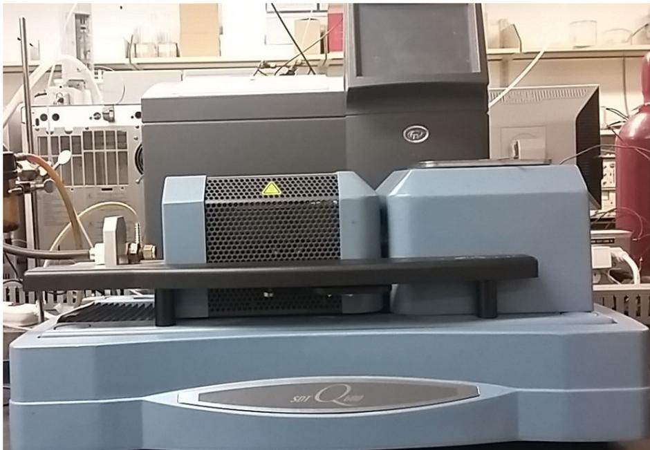
Figure 3.3 Thermo-Gravimetric Analyzer used
