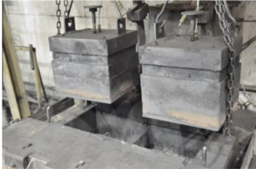
Figure 2.7 Sole-heated oven for semi-coke formation [MacPhee ,2013]
