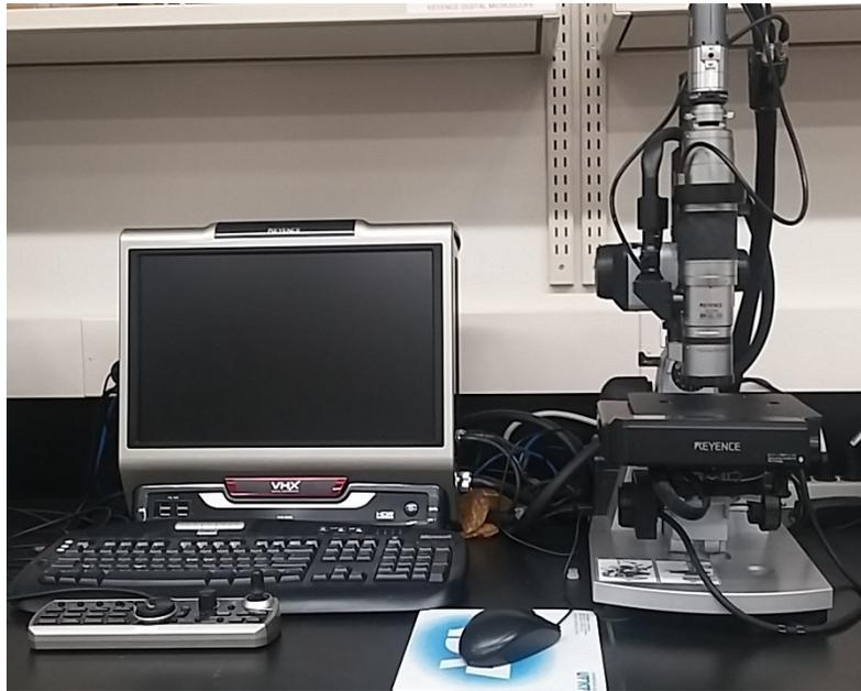
Figure 3.4 Keyence automated microscope used for image analysis
