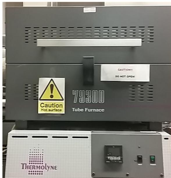
Figure 3.1 Horizontal Tube Furnace used for coal carbonization
