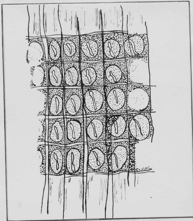
Figure 4. - Axis 25. Radial longitudinal section, showing the detail of the pits in the ray tracheid fields.
