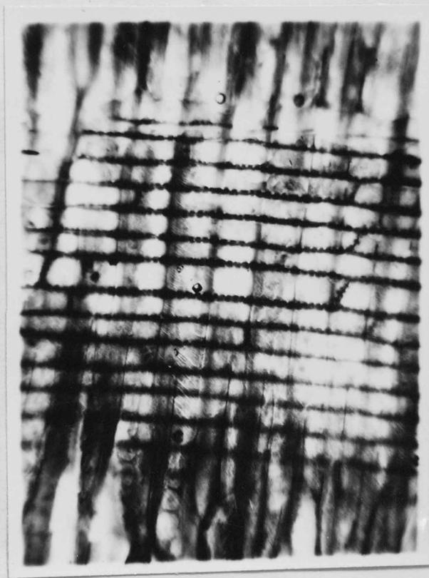
Plate XXI. - Axis 27. Radial longitudinal view of the medullary rays, showing the conspicuous "Abietinean thickening" on horizontal and cross walls. X 200.
