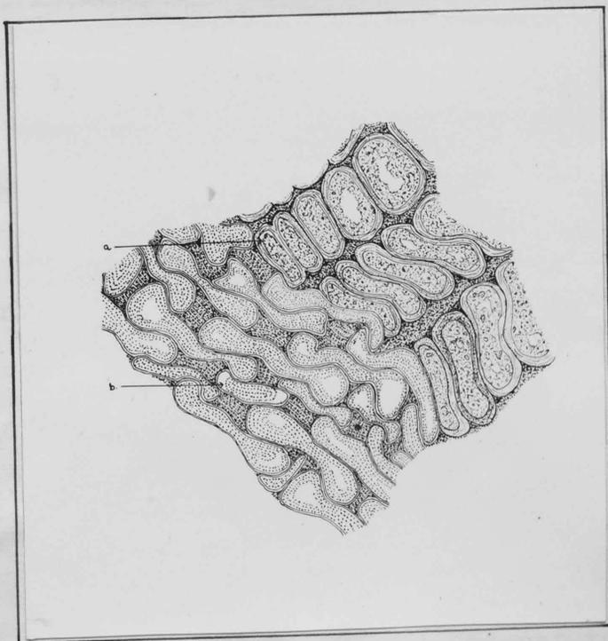
Figure 3. - Axis 25. Tracheid cavities filled with products of decomposition, and some shrunken from the cell walls as at (a) and (b).
