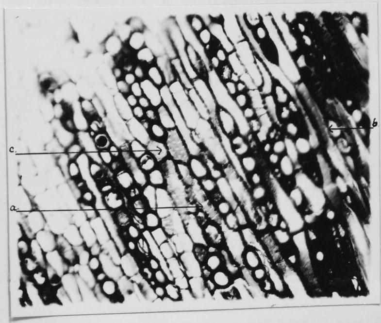
Plate XXVII. - Axis 27. Tangential longitudinal view of a zone of medullary ray hypertrophy showing probable sclariform pits at (a), the round simple pits of parenchymatous cells at (b) and the profusely pitted end walls of the medullary ray cells at (c). X 370.
