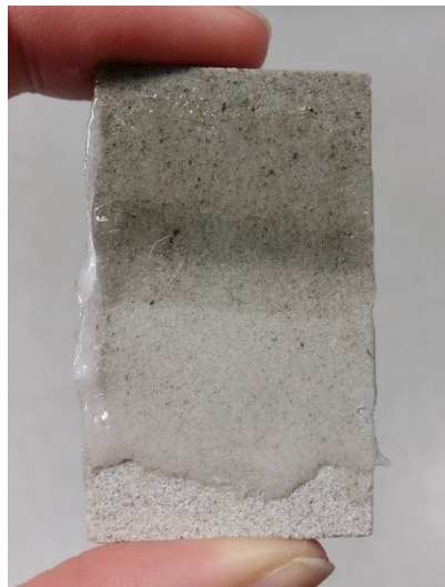
Figure 4.11 Berea rock coated with acoustic gel after an experiment
