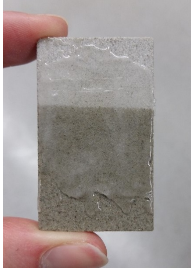
Figure 4.10 Berea rock partly imbibed with octacosane and coated with acoustic gel before an experiment
