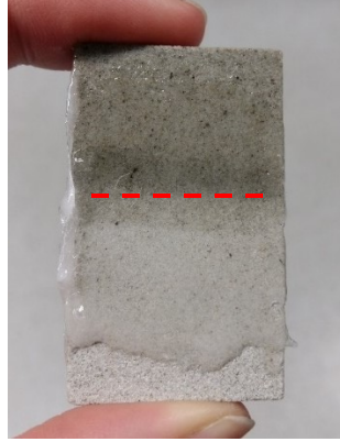
Figure 4.15 Section axis along which some of the rock samples were cut after an experiment with coating
