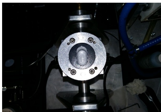
Figure 3.5 Acoustic cell containing solidified wax in the lower part – top view
